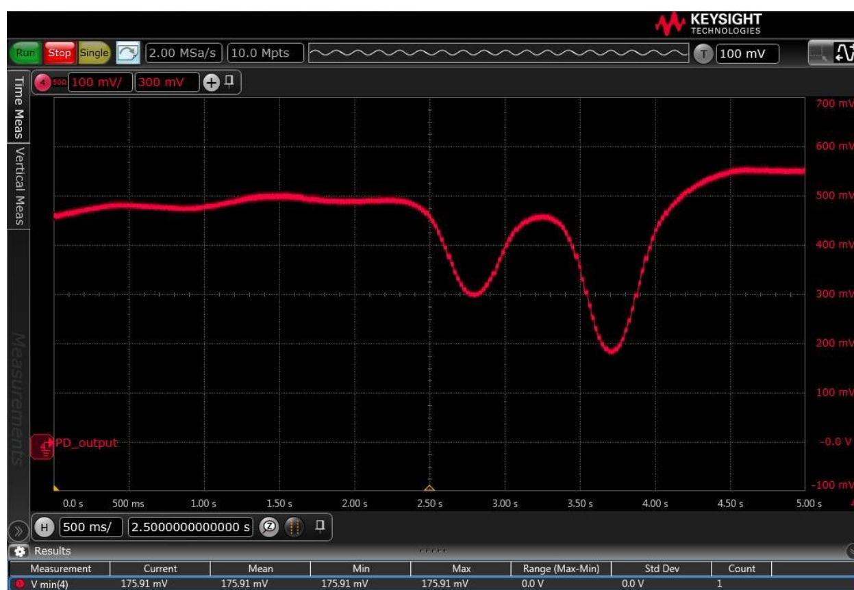
Figure 101. Photodiode response to increasing laser diode current showing both 5^2S_{1/2} \rightarrow 5^2P_{3/2} transitions. 14 \mu W optical power on cell.
