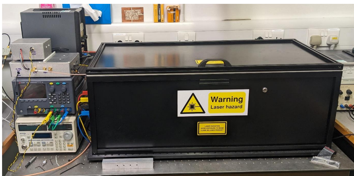
Figure 16. Safety enclosure used to encapsulate the experiment, with laser driver and power supplies to left.
