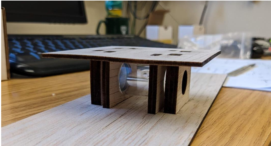
Figure 50. 85 Rb cell and 2x Thorlabs LA1270-B Plano-Convex lenses mounted in a balsa support structure.
