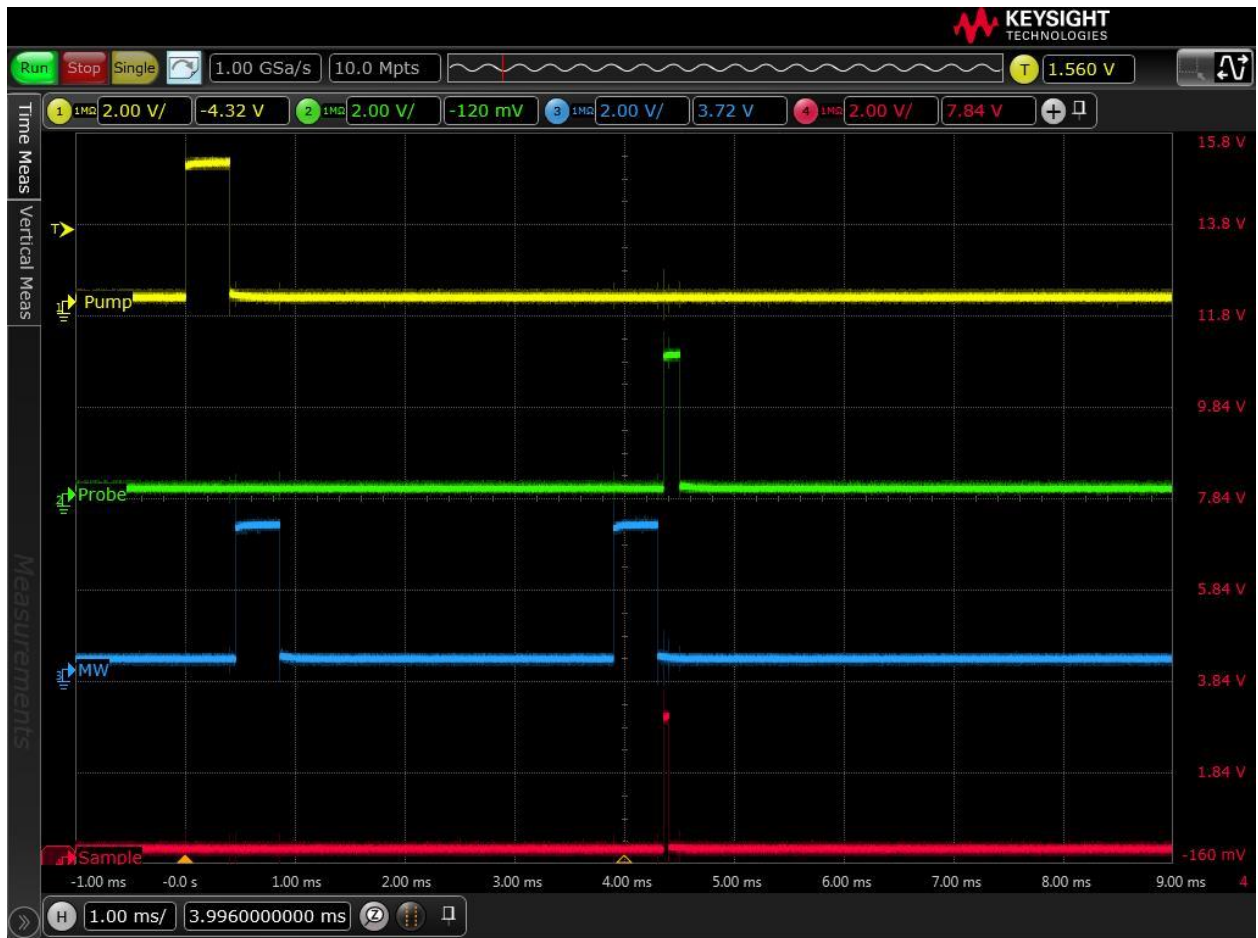
Figure 58. FPGA outputs as used to control a single POP cycle.
