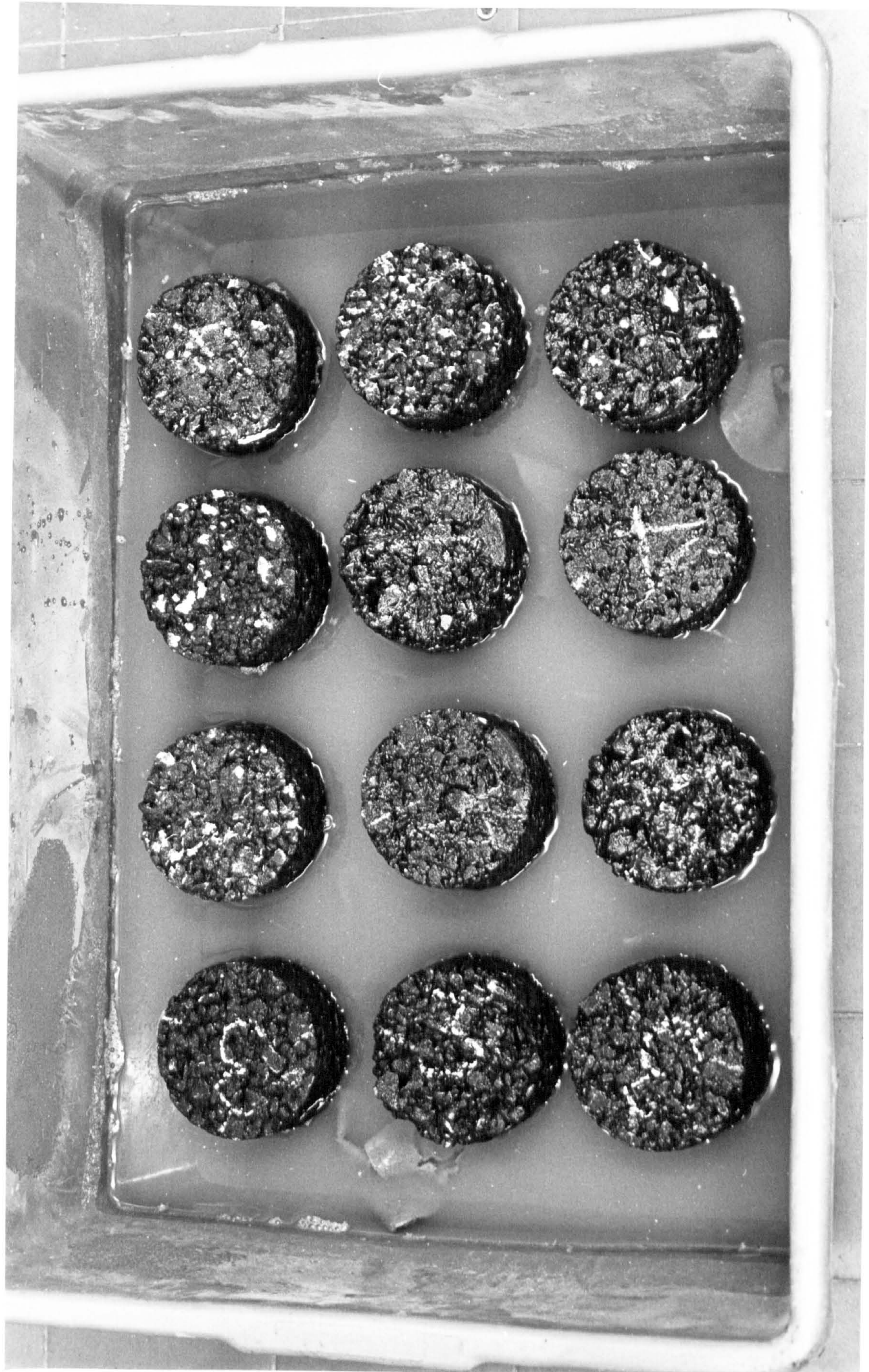
Plate 5.4 Capillary soaking test - specimen arrangement
