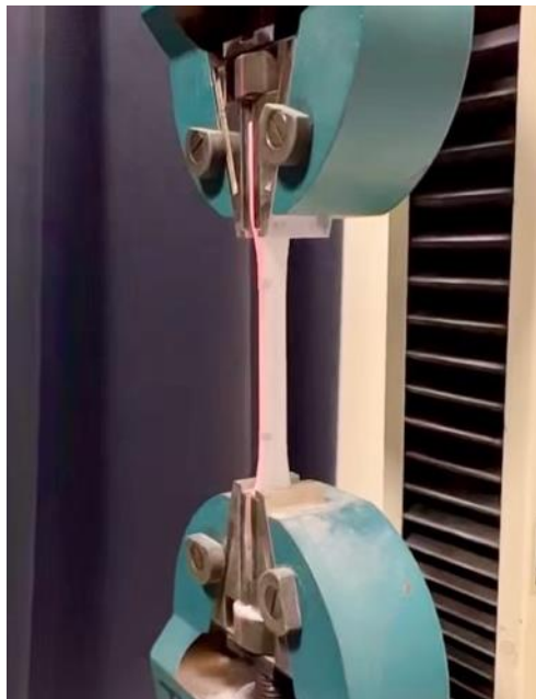
Figure 4.4 – A tensile specimen mounted between the grips of the Tinius Olsen H5KS tensometer used throughout this doctoral work.
