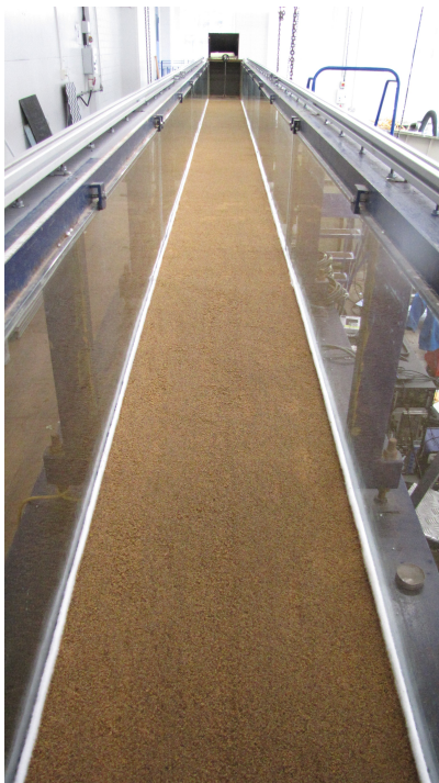
Figure 3.15: Sand foundation laid between section 4.8 m and the end.
