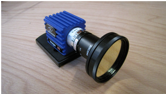
Figure 3.4: Imager MX 4M camera with a blue light bandpass filter used for PTV.
