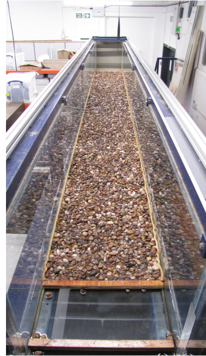
Figure 3.14: Initial section covered in gravel.
