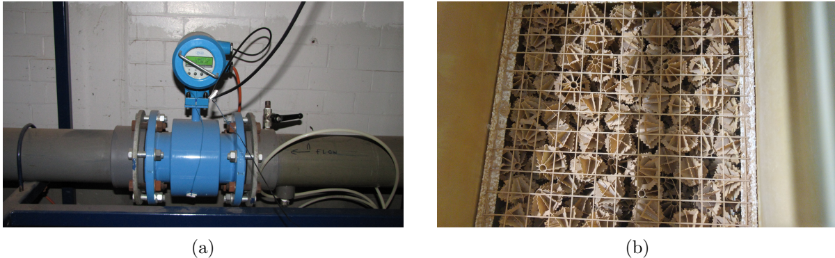
Figure 3.2: a) The in-line placed flowmeter. b) Porous elements used to break down inflow effects.
