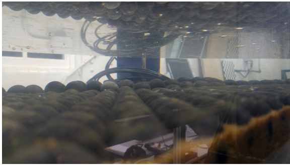
Figure 3.19: Example of bed failure.
