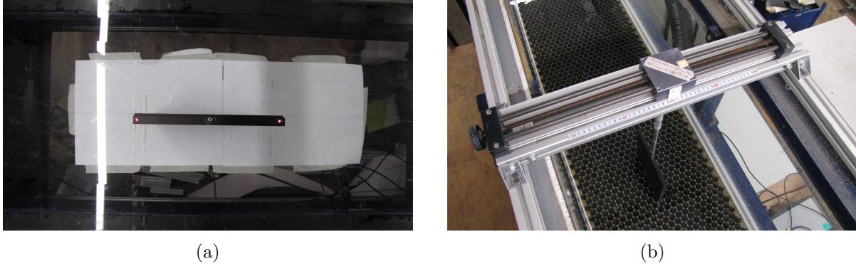
Figure 3.11: a) Alignment of the lasers for the PTV calibration plate. b) Traverse line mounting the PTV calibration plate.
