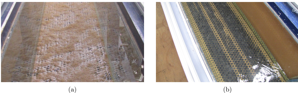
Figure 3.17: a) Sand sprinkled over the spheres for stabilisation. b) Waterworking of the composite bed in progress. Gradual removal of the excess of sand was observed.
