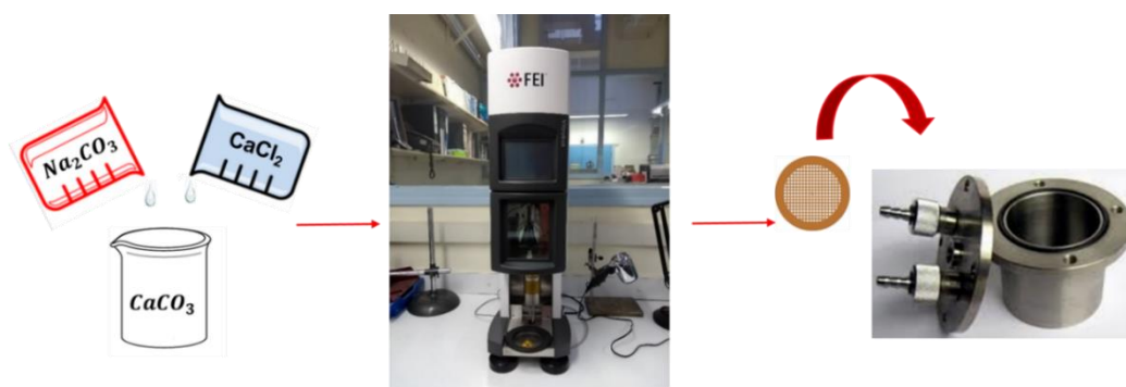
Figure 45 A schematic diagram of samples prepared by the plunge freezing vacuum-drying method.
