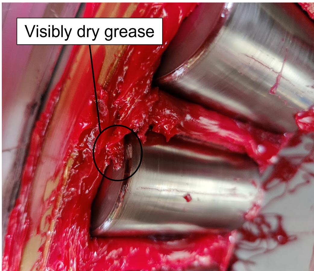
Figure 6.11: Picture of a dried grease clump next to the roller face-flange contact
