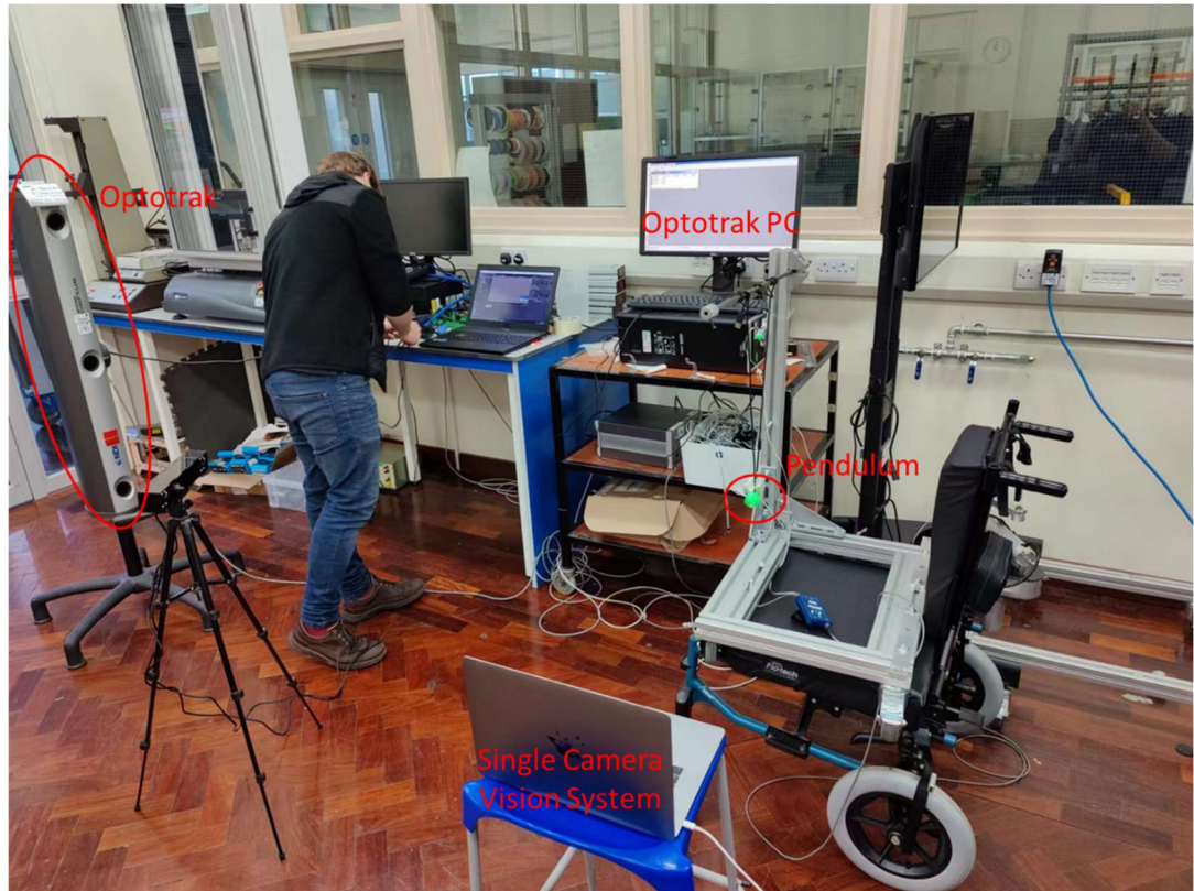
Figure 3.3 Single-camera based position tracking using a single pendulum.
