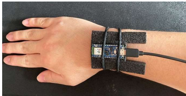
Figure 1: IMU sensor attached by two elastic bands on wrist
