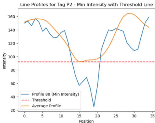
Figure 57: Particle ('P2') incorrect Sizing (interference)
