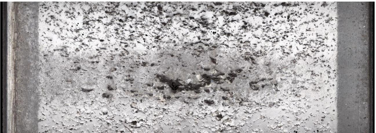
**Figure 5.7:** A close up of the surface feature observed using a Alicona infinite focus microscope after the water-lubricated twin-disc test was finished.
