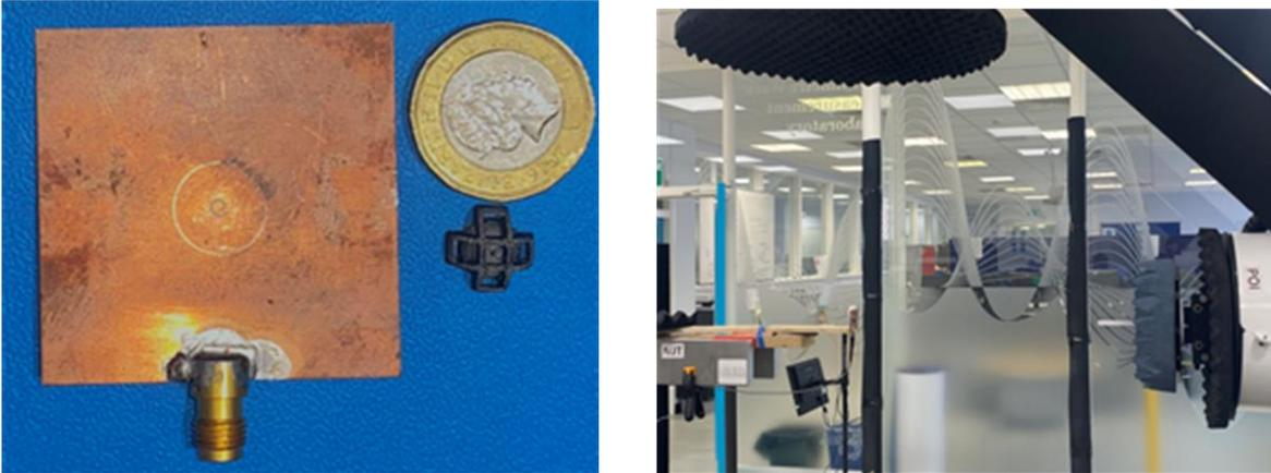
Figure 5.32: The prototype of the proposed hemispherical DRA with a perforated dielectric coat.
