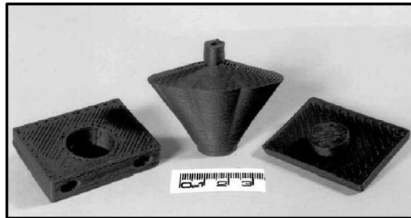
Figure 2.15 3D printed parts by FDM metal technology using the iron/nylon filament [38].
