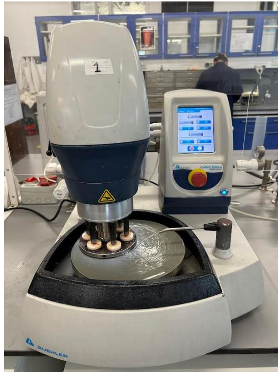
Figure 4.30 The polishing machine containing a six-specimen holder.
