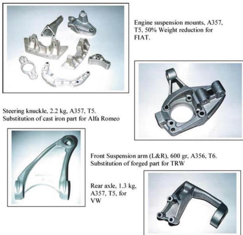
Figure 3.19 Demonstrate some automotive parts produced by SSM processing using MHD route [23].
