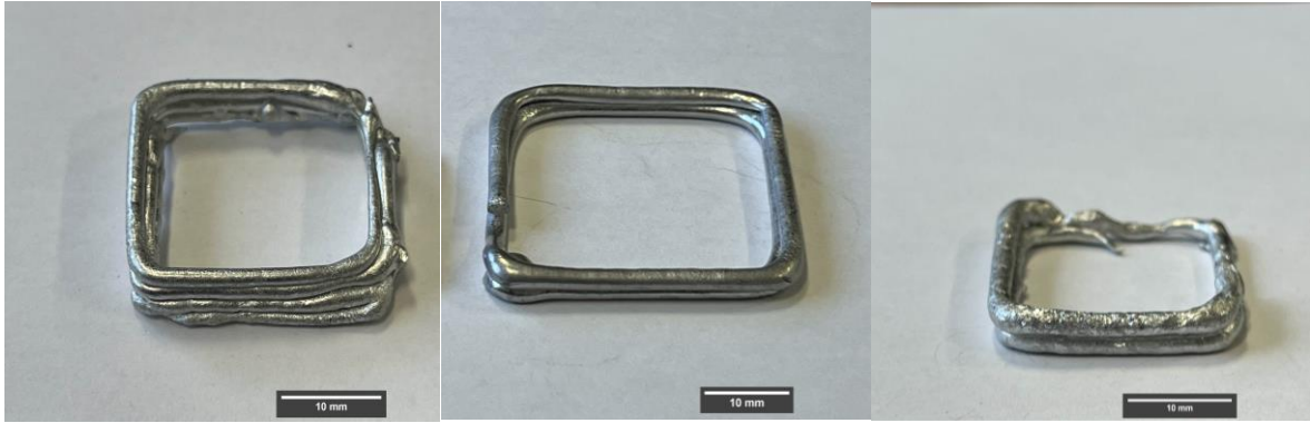
Figure 6.18 Demonstration of deposited multilayer of the Zn-40Sn alloy at ambient bed temperature.
