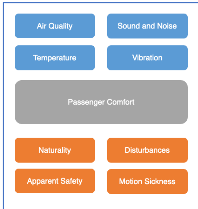
Figure 1.9. Factors influencing ride comfort in traditional (blue) and automated (orange) vehicles. Redrawn from Elbanhawi et al. (2015).
