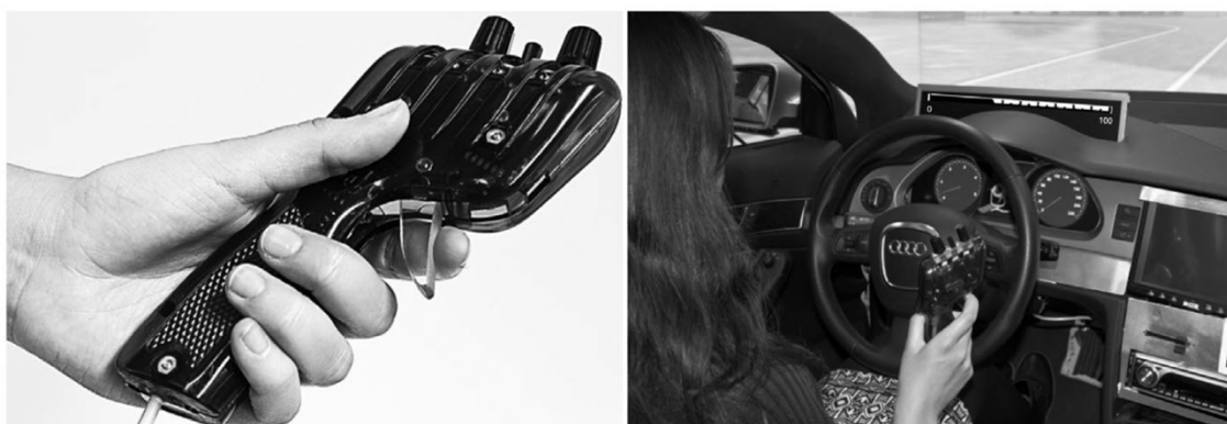
Figure 1.4. Handset used for the online assessment of comfort during automated driving in a driving simulator (Dettmann et al., 2021; Hartwich et al., 2018).
