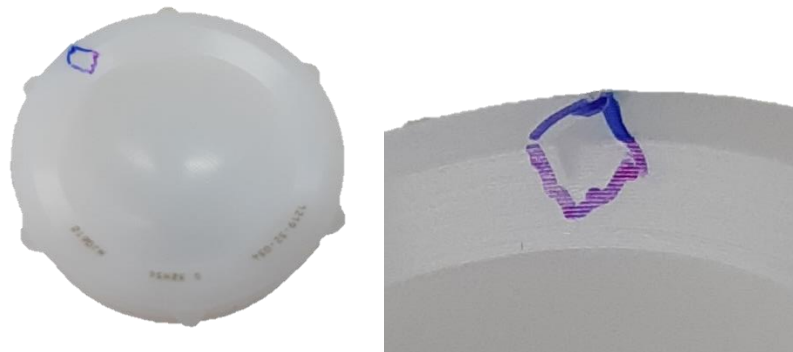
Figure 3.2. A polyethylene liner subjected to 40 000 cycles of impingement loading. (A) Impingement loading generated a diamond shaped deformity on the liner edge spanning a portion of the chamfer and top surfaces. There were no visible signs of fatigue damage (e.g. cracking or delamination).
