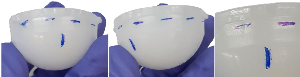
Figure 7.7. Signs of plastic deformation (not characterised by CMM) were visible on the backside of the liners (underlined in blue). The vertical blue line was positioned superiorly on the liner.
