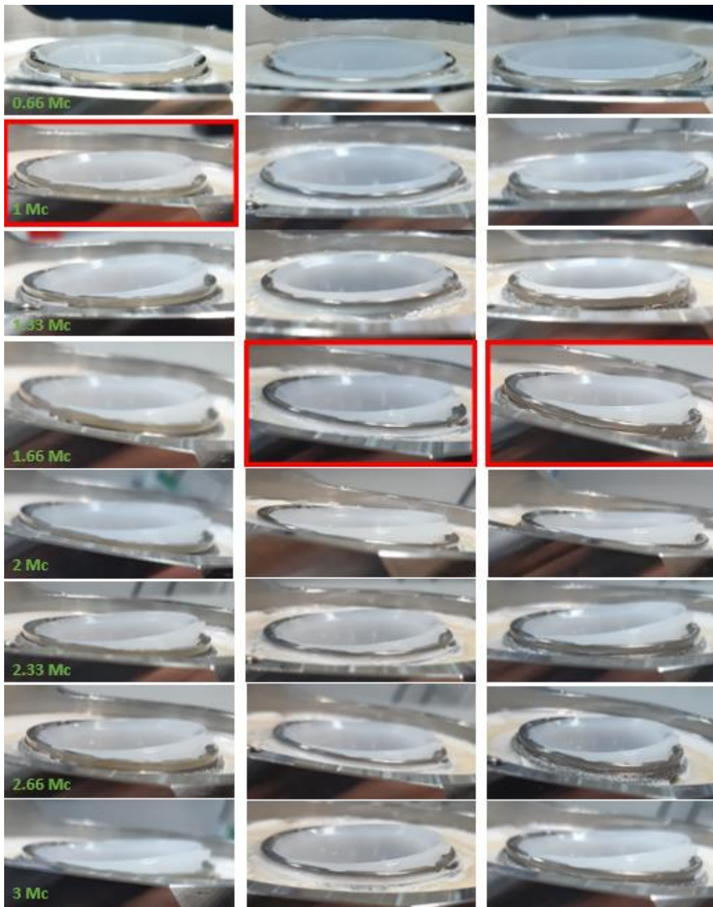
Figure 7.3. Photographs displaying the relative positioning of the liners within shells at measurement points from 0.6 Mc to the end of the test. Red rectangles highlight the incidences of adverse deformation events in each liners (see also Table 7.1). Either side of these events, no substantial changes in liner positioning or seating were visually identified. The edge loaded superior side of the liner is located on the left of the photos.
