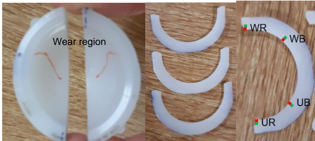
Figure 5.4. Three sections were cut superiorly through the liner. Cube specimens were prepared from the bearing surface (B) and the liner rim (R) at worn (W) and unworn (U) regions of each section. The sub-surface specimens (green) were taken approximately 1 mm below the surface specimen (red).
