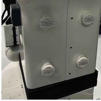
Fig. 5.45 The Bluetooth beacons deployed on TIAGo.
