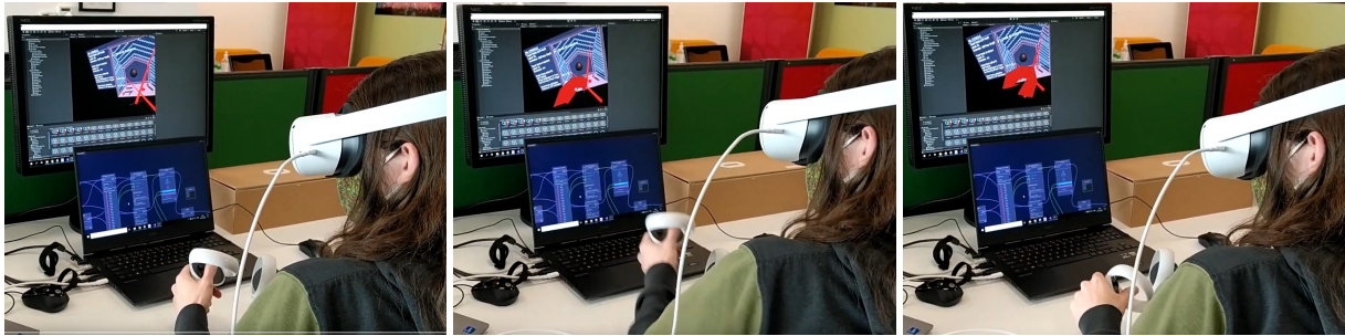
Figure 109: A participant records additional movement data for his movement interactions. He implemented a red trail to visualise in real-time what the window of features ‘sees’ from his movement. In the pictures the trail can be seen ‘growing’ as he makes the gesture. In the end the trail will disappear matching the sample size of the window of features.
