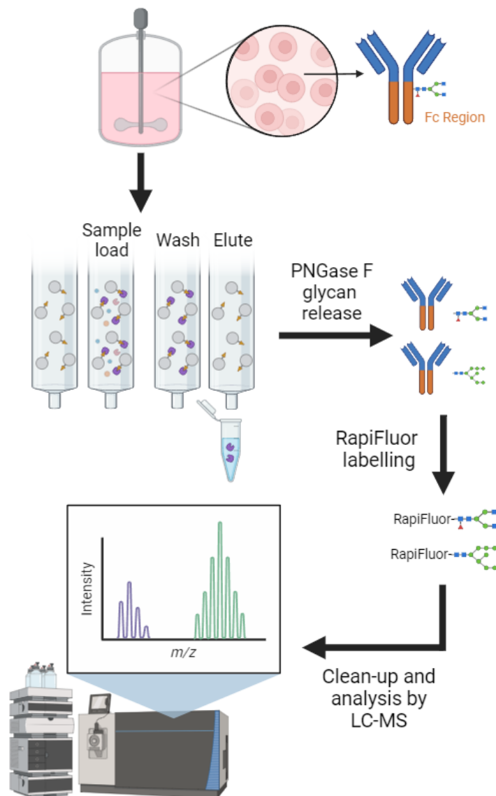
Figure 2 - mAb purification and glycan profiling workflow. Samples are taken from bioreactor cultures and mAbs are purified using protein A columns. Glycans are released from mAbs by PNGaseF and labelled with RapiFluor. The RapiFluor glycans are then detected by LC-MS. Diagram created with BioRender.
