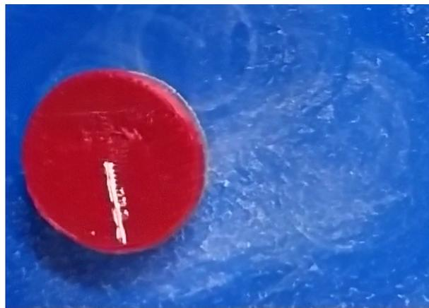
**Figure 5.1:** Circular patterns of the polished acrylic surface by actuating the lapper on it for 1 min.
