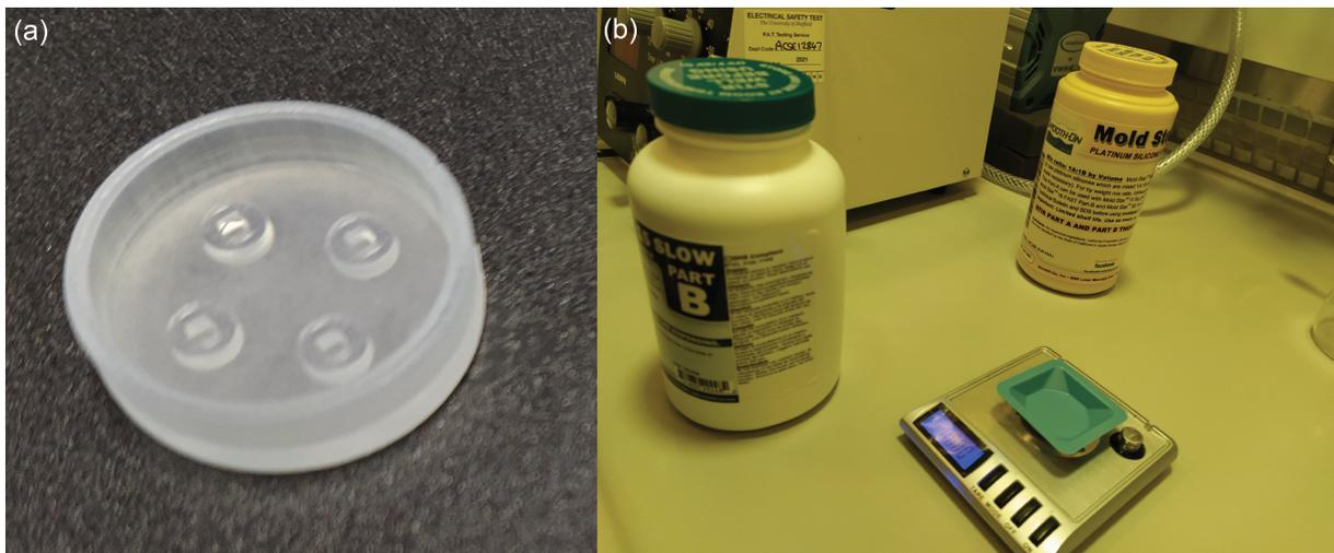
**Figure 3.10:** (a) 3D printed mould used for mould-making using soft-lithography.(b) Mold Star Parts A & B prepared to pour into mixing dish placed onto a precision scale
