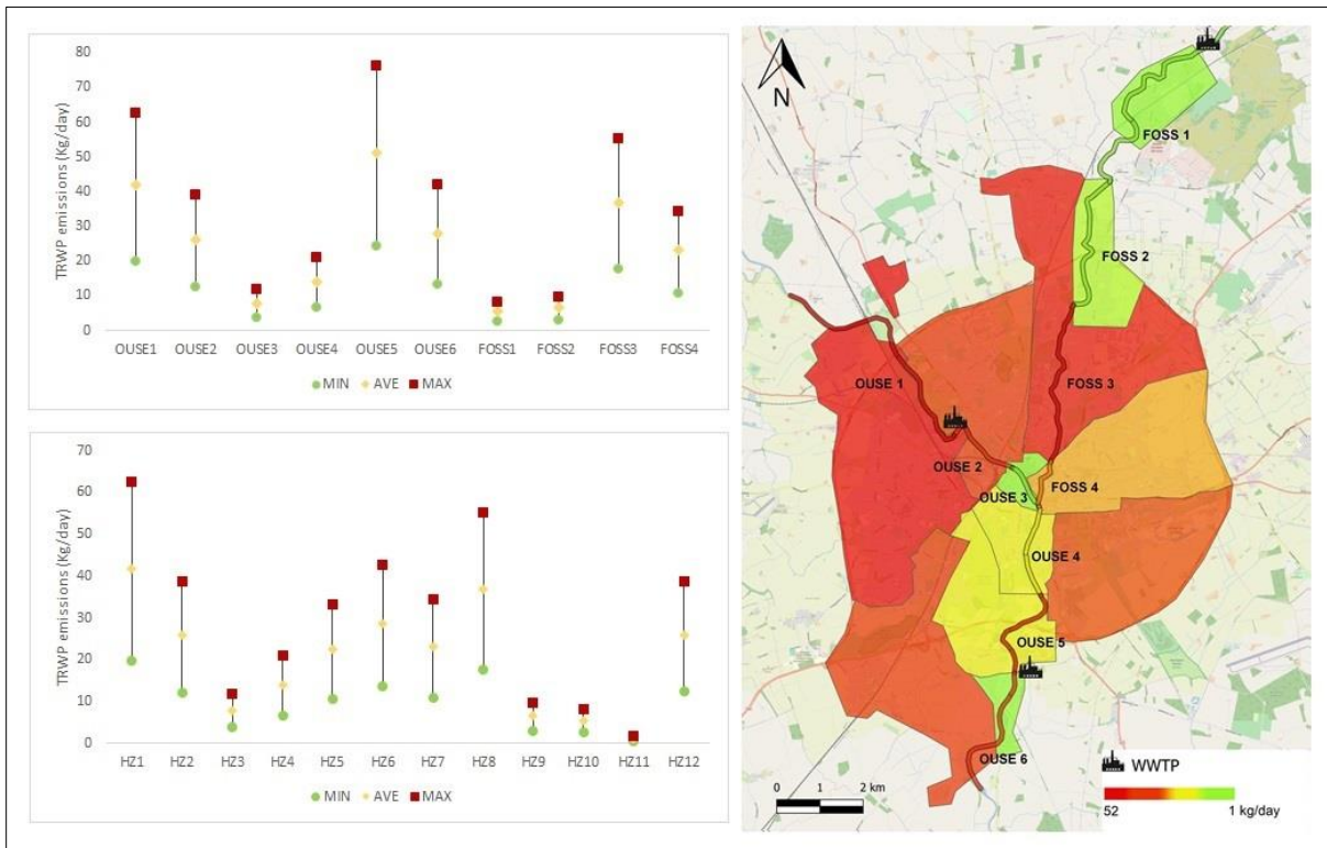
Figure 2.8. Mean daily emissions of TRWP to York's river sections (OUSE1, OUSE2, OUSE3, OUSE4, OUSE5, OUSE6, FOSS1, FOSS2, FOSS3 and FOSS4) and hydrological zones for the three simulated scenarios minimum (MIN), average (AVE) and maximum (MAX) including a map of mean emission values per day with the HZs and RSs for the average scenario.
