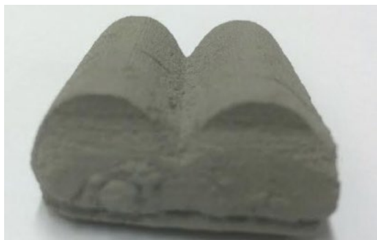
Figure 2.9: A binder jetted of 420 stainless steel components (29).
