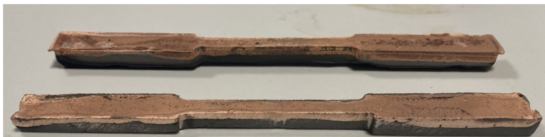
Figure 8.4: The tensile test coupons fabricated under the specifications outlined in the BS EN ISO 6892-1:2016 Standards. These specimens have been prepared to undergo Ultimate Tensile Strength (UTS) testing.
