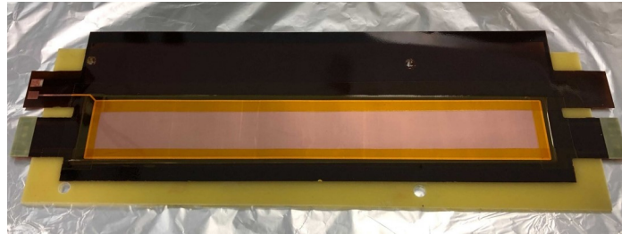
Figure 5.2: The \mu -RWELL detector used for the test chamber studies with visible active area.
