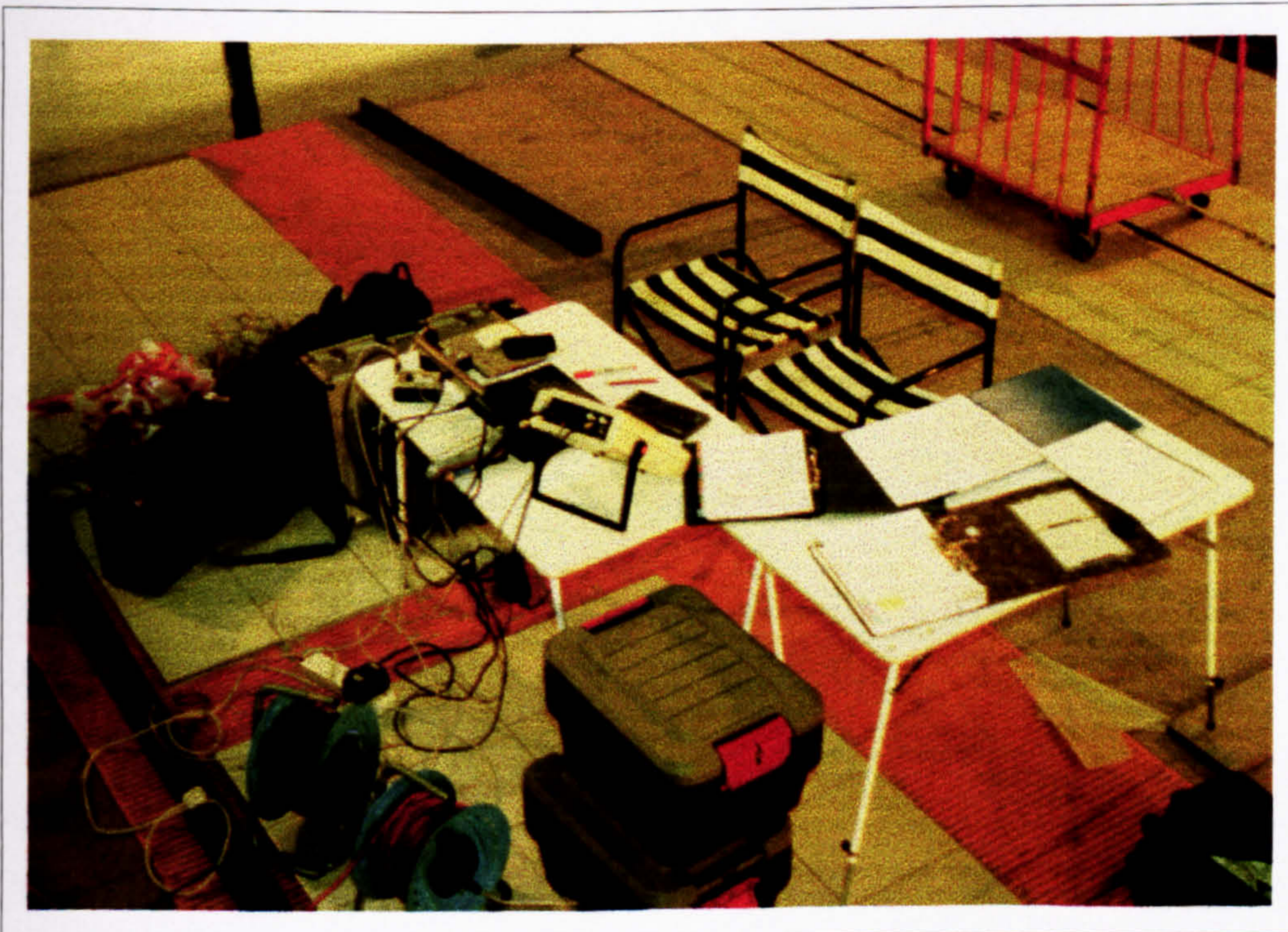
Figure 5.45: Structure B (Uncracked) - Limited equipment, consisting of a dual-channel spectrum analyser and portable PC (for in-situ parameter estimation), used for field testing of this structure.
