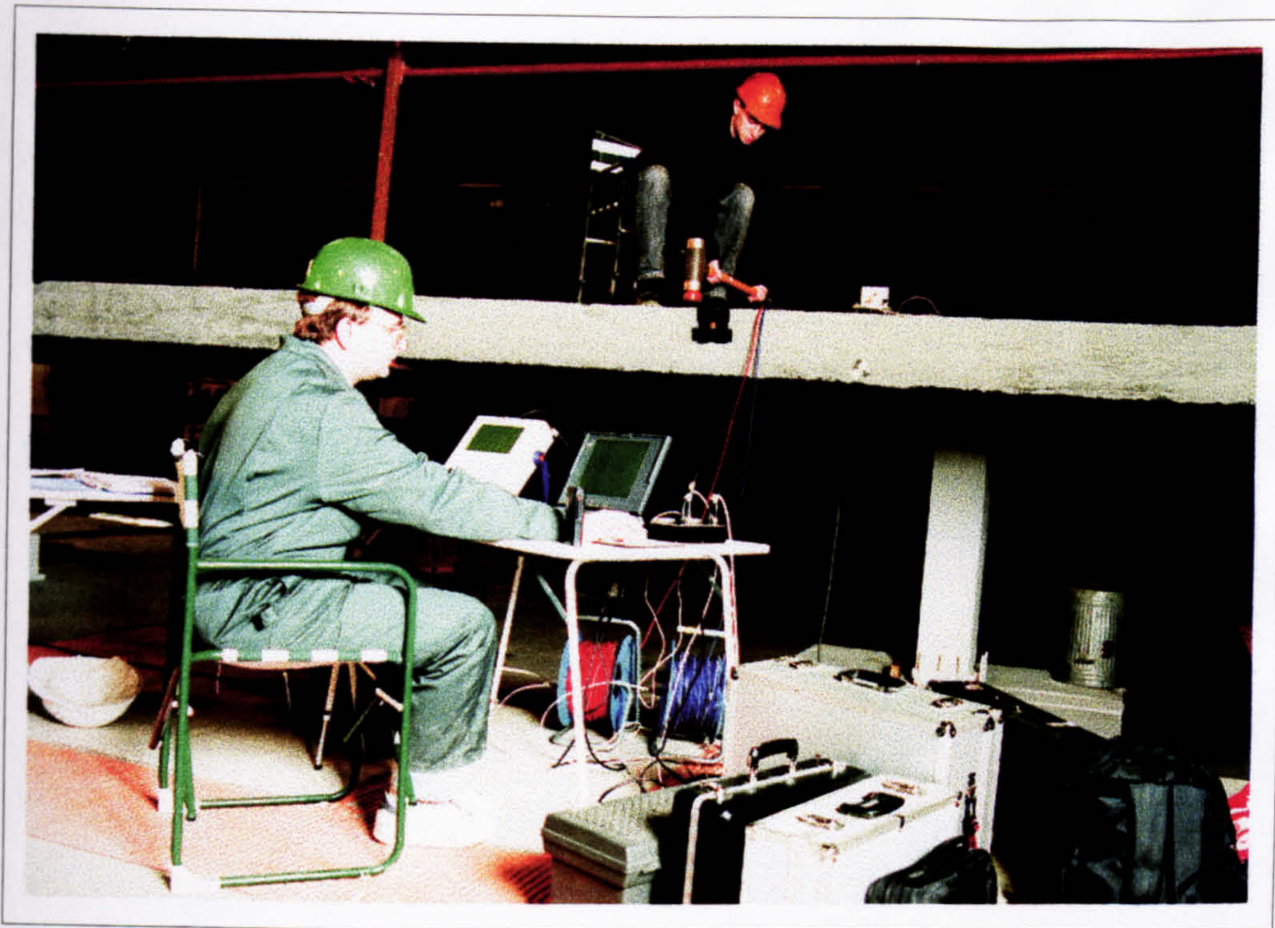
Figure 5.46: Structure B (Uncracked) - Hammer excitation and data acquisition.
