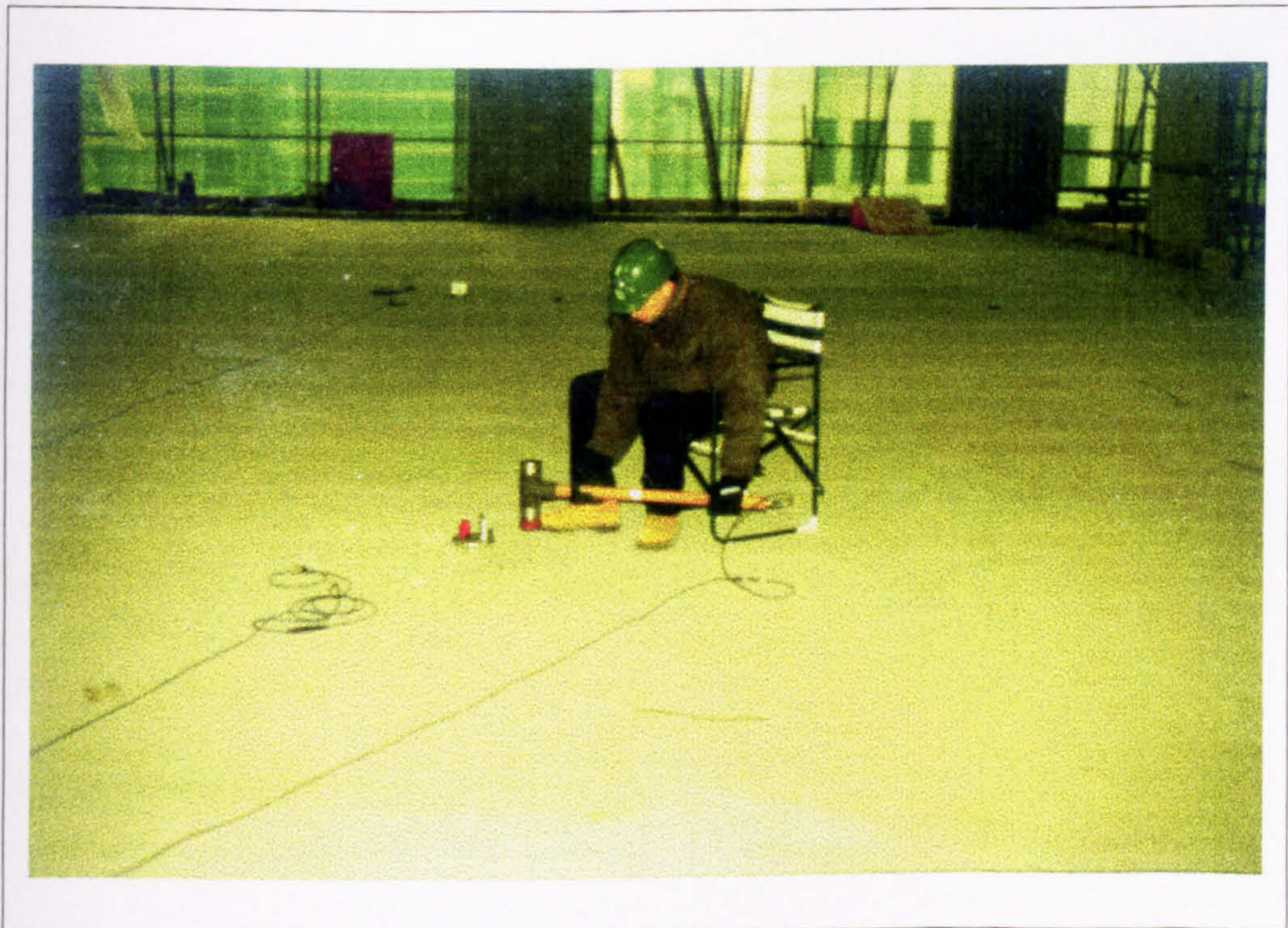
Figure 5.71: Structure C (Unclad) - Hammer excitation at TP35.
