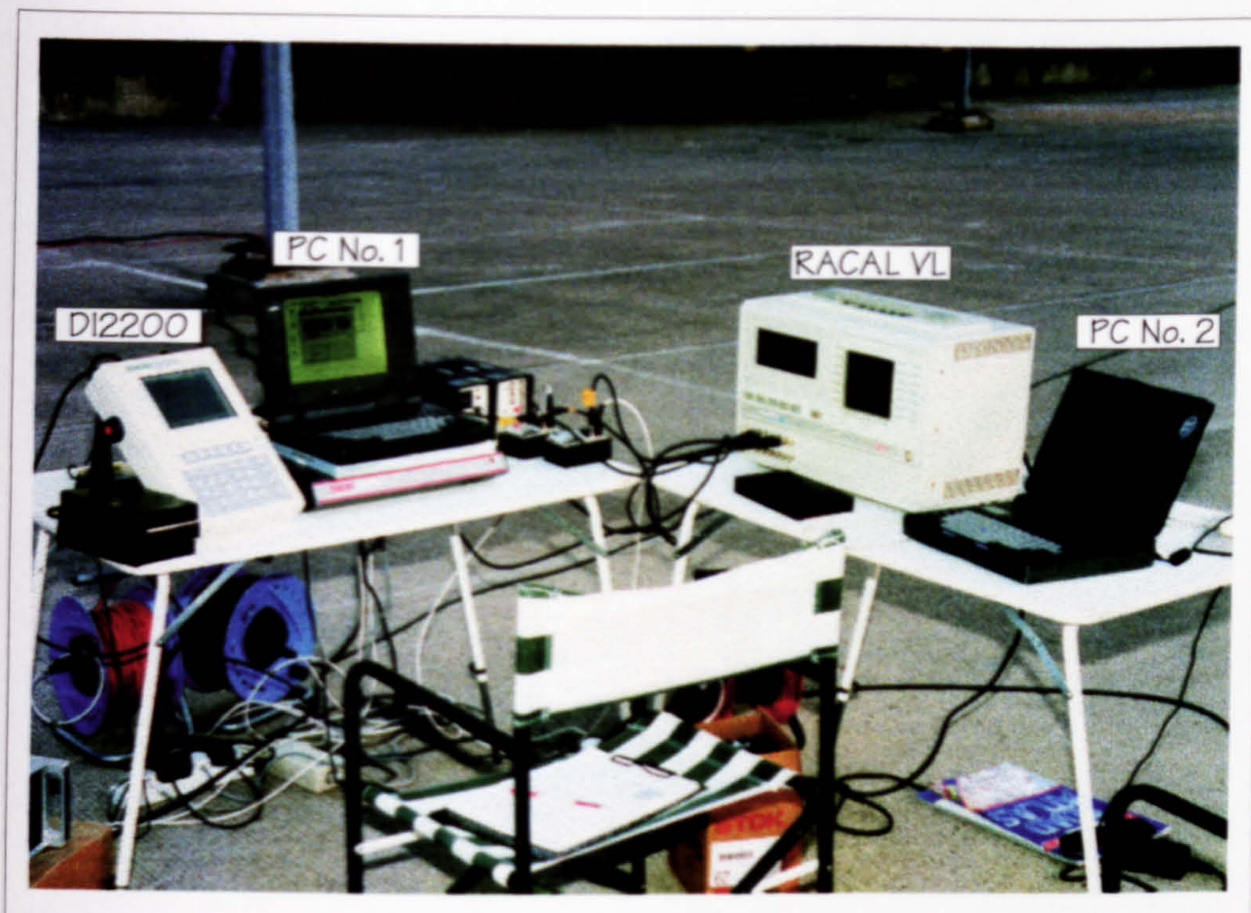
Figure 5.91: Structure D - Hardware used for data acquisition.
