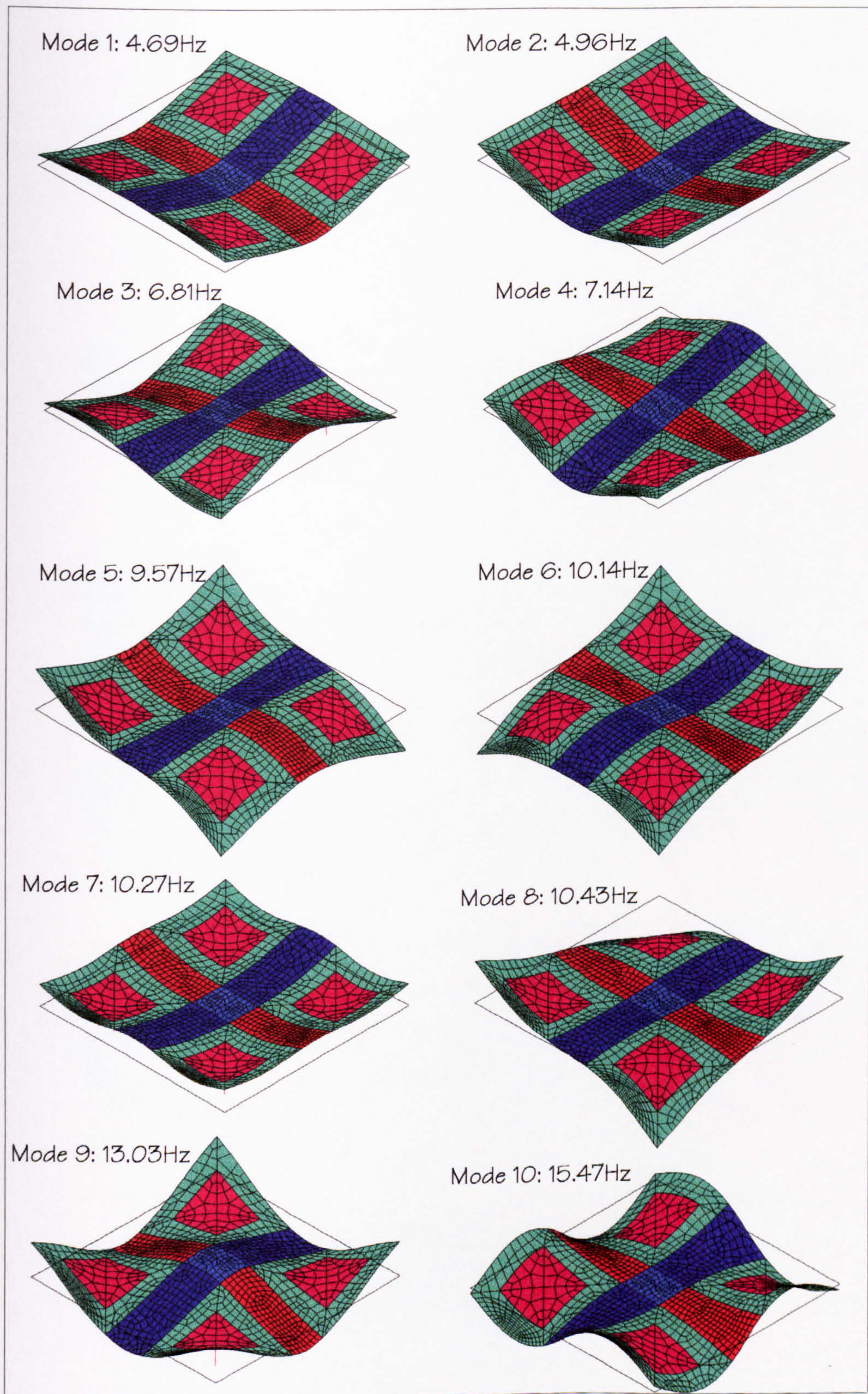
Figure 6.22: Structure B (Cracked) - The analytically calculated mode shapes and natural frequencies.
