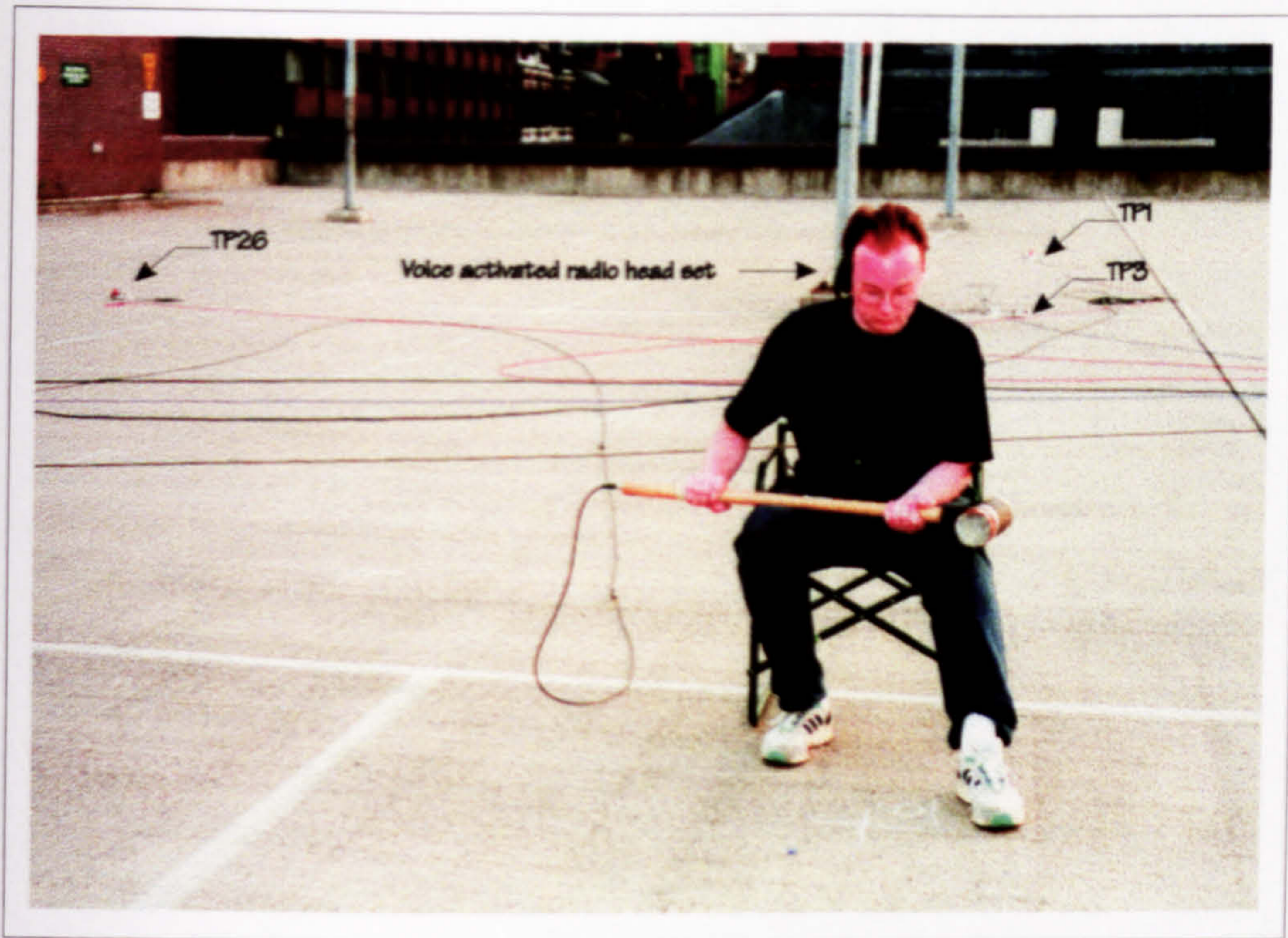
Figure 5.93: Structure D - Hammer test operator receiving instructions via the hands-free voice-activated two-way radio head set.
