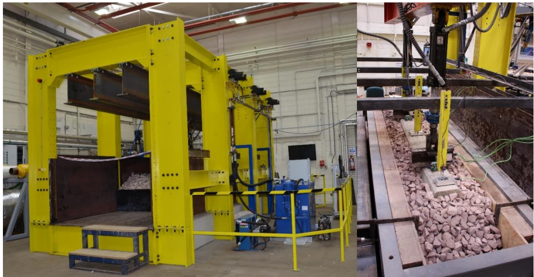
Figure 3.19 Full scale ballast testing
