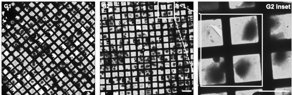
Figure 4.12: Cryo-EM Atlas maps depicting two optimal grids selected for subsequent cryo-FIB milling.
