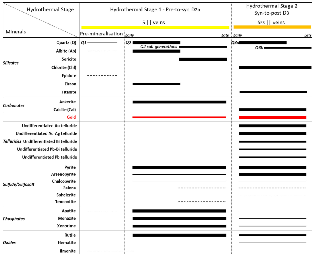
Figure V.15 – Mineral paragenetic sequence for the Argyle deposit. SF3 || = veins parallel to the axial planes of F3 folds.
