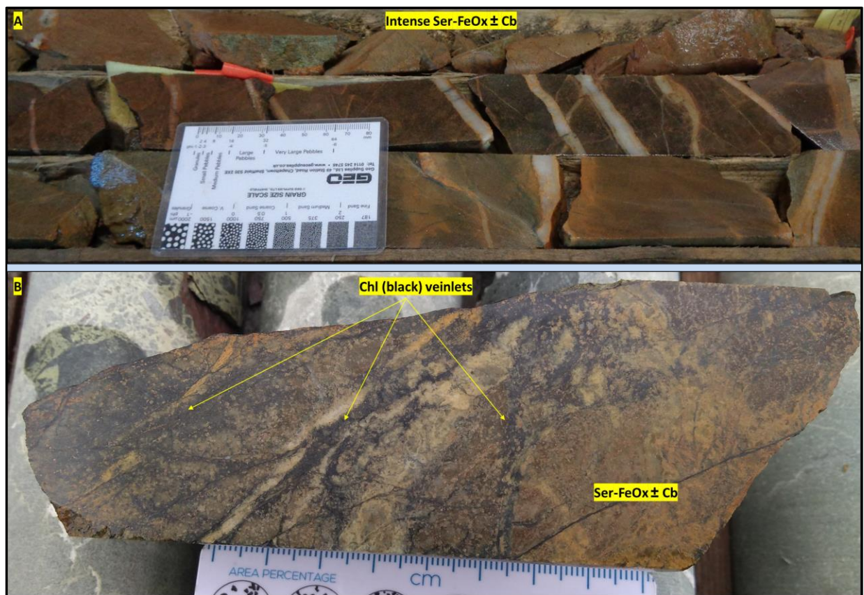
Plate V.18 (above and next page) – Representative images for the proximal and the outer alteration halos observed in the Juliet area: A – Intense, orange-brown alteration halo composed of sericite, iron oxides (FeOx), and to a lesser degree carbonates, drill hole RJ-00-06; B - Intense, orange-brown alteration halo composed of Ser-FeOx \pm Cb, crosscut by chlorite (black) veinlets; C – Grey-cream alteration composed of Ser-Cb crosscut by Qtz-Chl and Chl (black) veins; D, E – Outer alteration halo characterized by epidote \pm quartz-carbonate veins associated with yellowish green (epidote-chlorite) pervasively altered basalts; F, G – Hand specimens of least altered basalts from the Juliet South zone - massive, fine grained, weakly silicified basalt ( F ) and fine grained, locally variolitic, weakly epidote altered basalt ( G ); C, B, D, E – drill hole RJ-00-08.
