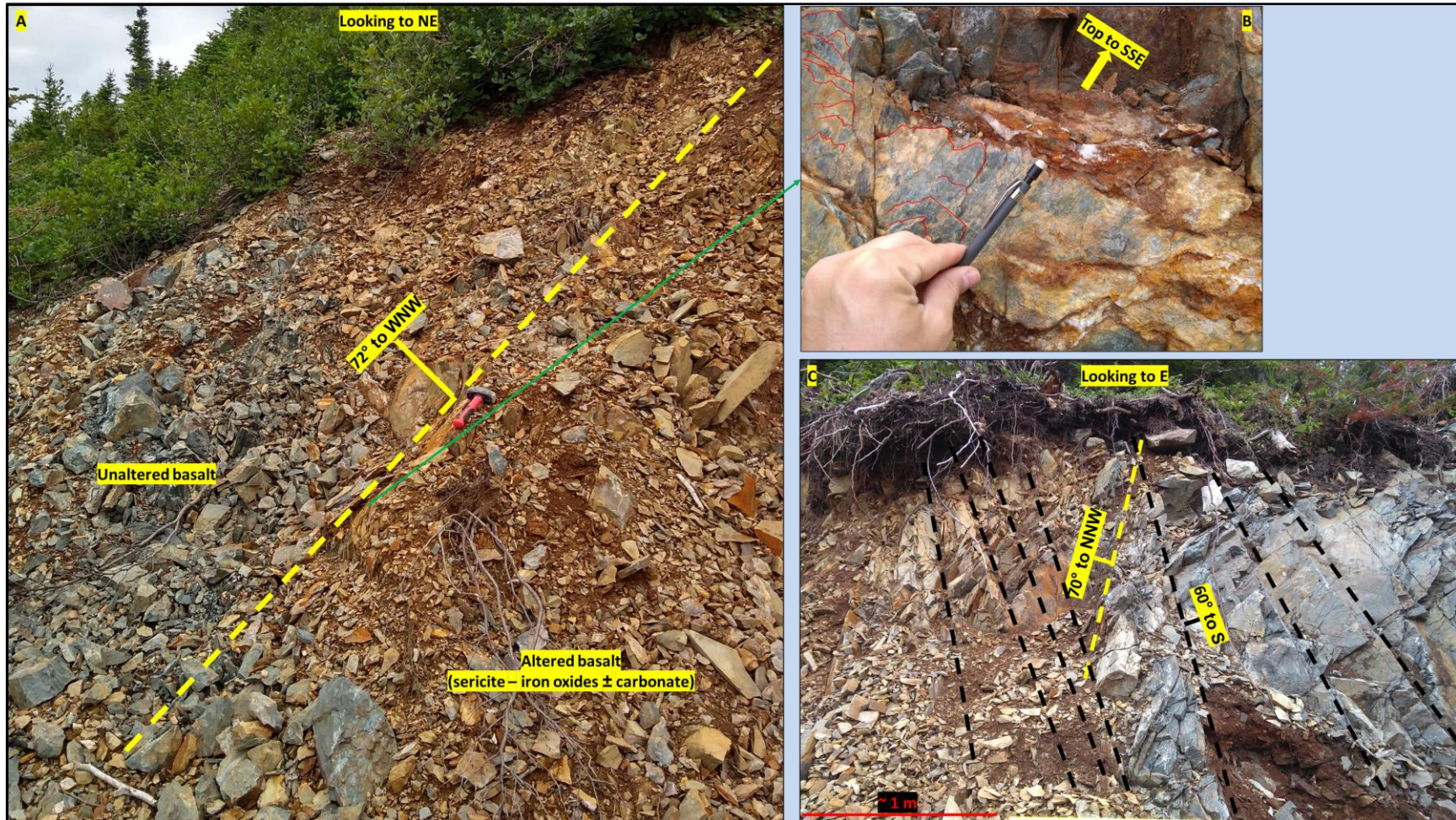
Plate V.16 – Representative images for the main structures that affect the Juliet South zone: A – Contact (traced by the yellow dashed line) between unaltered basalts and intensively altered basalts in the northern part of the Juliet North zone, note the contact corresponds to a D_{2b} fault that accommodates a hanging-wall (top) motion to SSE ( B ); C - Contact (traced by the yellow dashed line) between intensively altered basalts and unaltered basalts in the southern part of the Juliet North zone, note the syn-to-post D_4 south dipping faults (black dashed lines) that overprint the contact (probably a D_{2b} structure).
