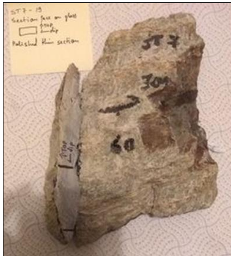
Figure III.4 - Example of an oriented sample cut perpendicular to the foliation and parallel to the stretching mineral lineation, note the location of the future section plane marked on the cut surface and the top and the dip marks.
