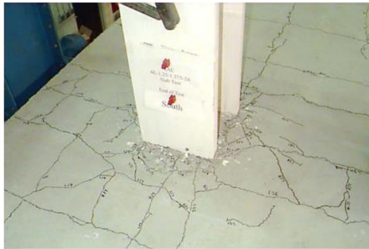
(b) View of Composite Slab Around Column
