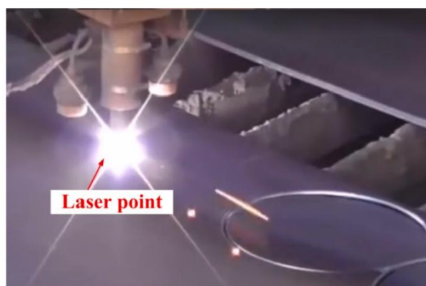
Figure 2.20: Laser cutting of web opening (Qiao, Guo, et al., 2022).
