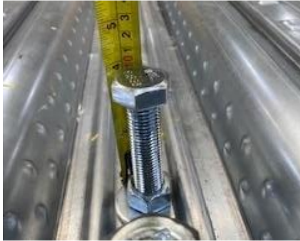
Figure 4.2: The height of the bolted shear connector above the top beam flange (mm)
