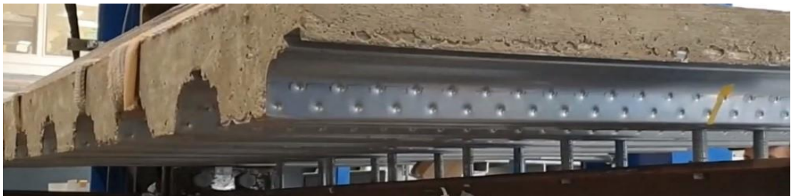
Figure 4.14: Disconnecting the composite slab of the solid specimen to be reused for the next test.
