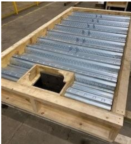
Figure 4.3: Shuttering of test specimen.
