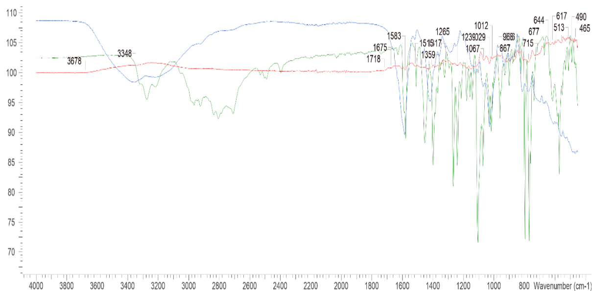
Figure 149. FT-IR spectra comparison of DBS-CONHNH 2 /Alginate xerogel beads (blue) containing 0.4% (wt/vol) DBS-CONHNH 2 and 1% (wt/vol) alginate, propranolol HCl dry powder (green), and propranolol loaded DBS-CONHNH 2 /Alginate xerogel beads (red).
