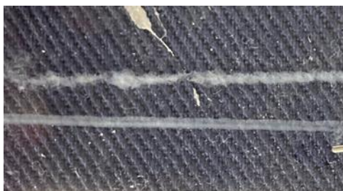
Figure 89. 3D printed 1.5% (wt/vol) DBS-COOH. Top line (Needle size 26G, rate of 5.1 \mu\text{L}/\text{min} ), bottom line (Needle size 23G, rate of 3.4 \mu\text{L}/\text{min} ).
