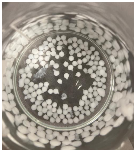
Figure 43. BG-C12/Alginate hybrid beads (composed of 0.35% (wt/vol) glutamine-C12 with equimolar benzaldehyde, and 1% alginate) in a water bath.
