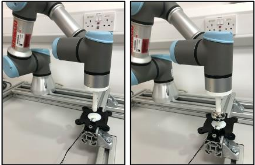
Figure 52 – Sensor verification experimental original setup (LEFT) including a 3D printed stem component (with fitted magnet) mounted to a UR3 robot arm position above an mlx90393 Triaxis magnetometer sensor held in a 3D printed mount and the same setup fitted with a metal femoral head (RIGHT).
