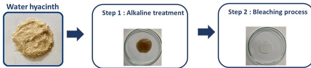
Fig. 56 Diagram of chemical pretreatment of water hyacinth
