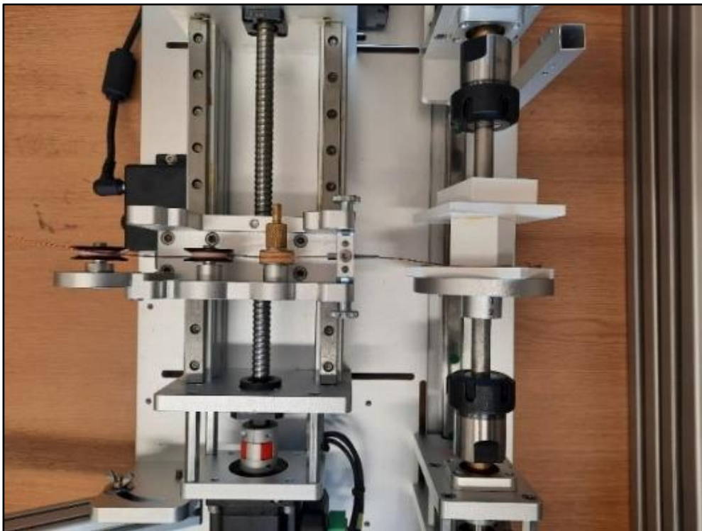
Figure 3.7. (a) Linear winding machine used for experimentation model "CNC Coil Winder MK4"
