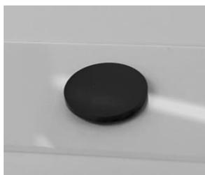
Figure 5.34 Oxygen deficient LST after reducing in 5% H<sub>2</sub>/N<sub>2</sub> gas.
