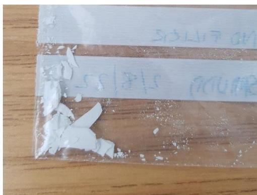
*Figure 5.24 Image of cold sintered and annealed pellet with no filler which was mechanically unstable.*
