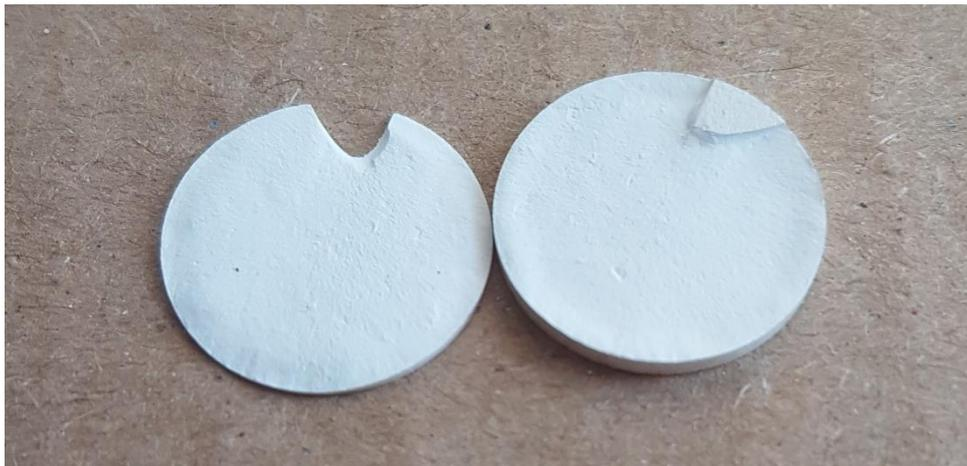
*Figure 5.20 Cold sintered and annealed pellet through-thickness split.*
