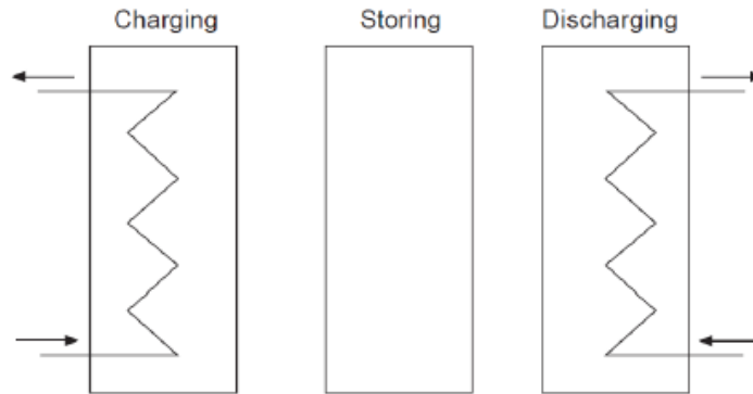
Figure 2.10: Schematic of a thermal energy storage cycle [97].
