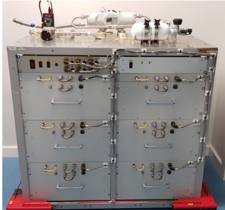
Figure 2.5: Son of whole air sampler in an aircraft. Source: SWAS TSSE [69].
