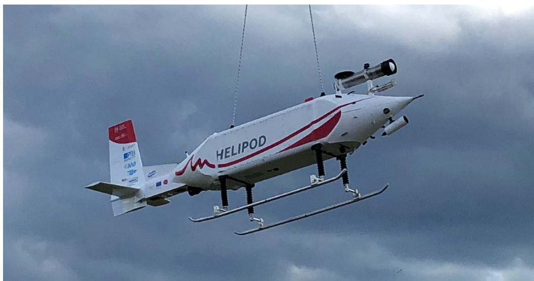
Figure 2.20: DLR's helicopter towed probe HELiPOD during take off.
