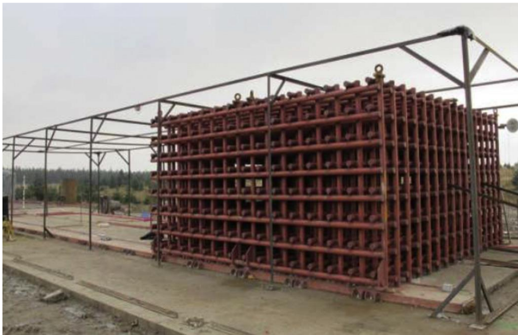
Figure 6.1. The congested rig of Shell large scale test in the frame of 20×6×3 m [21].
