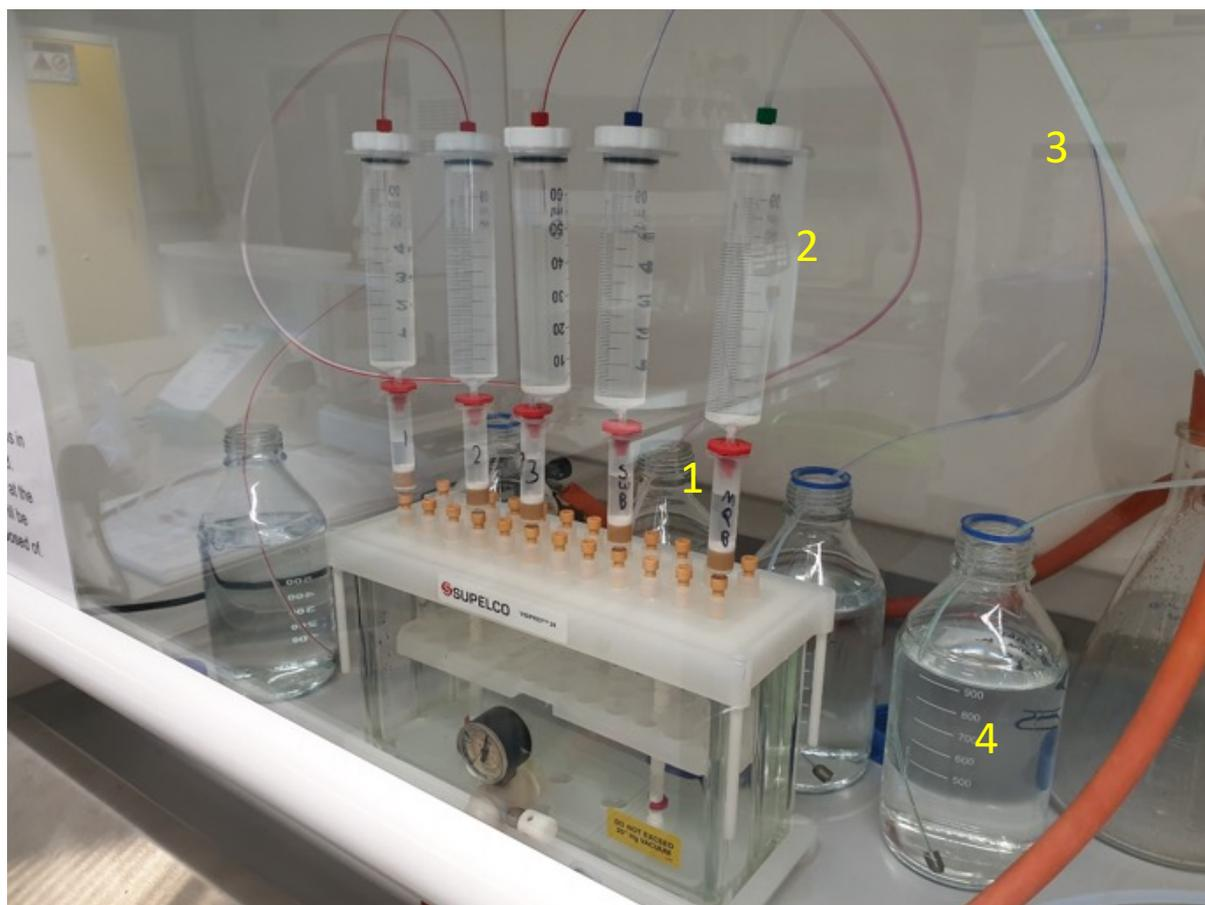
**Figure 5** - Apparatus used for solid phase extraction. The number labels correspond the following components: **1** is the PPL SPE cartridge; **2** is the reservoir for the sample; **3** is the tube used to fill the reservoir with the sample and **4** is the sample itself.
