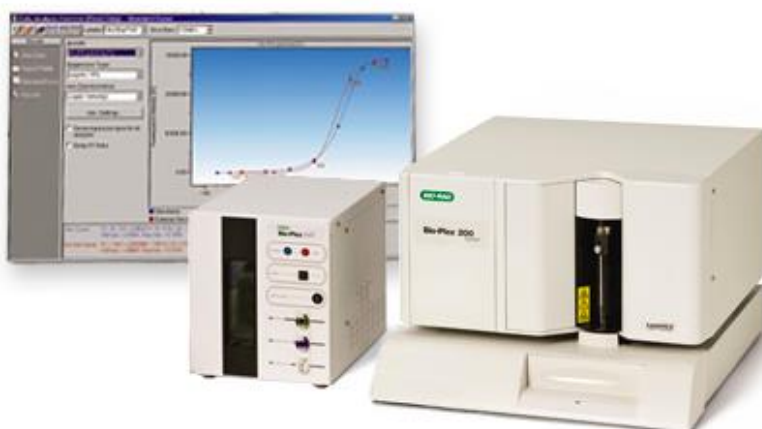
Figure A2.3.3 - Bio-Plex ® 200 System used to measure the fluorescence
