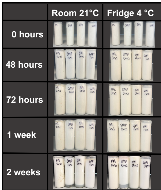
Figure 22. Photographs showing 0h, 48h, 72h, 1 week and 2-week storage of protein emulsions. Left column shows storage 21°C, right column shows storage at 4°C.
