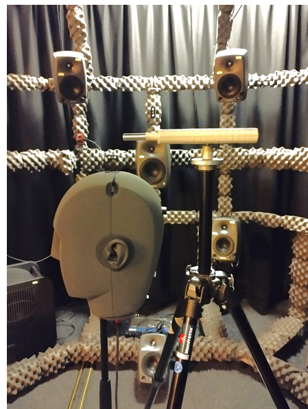
Figure 5.20: KU100 dummy-head side view, with Sound Level Meter on top.
