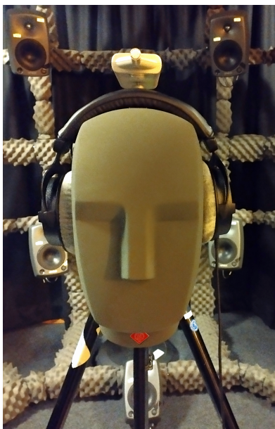
Figure 5.19: KU100 dummy-head on front view, with Sound Level Meter on top.
