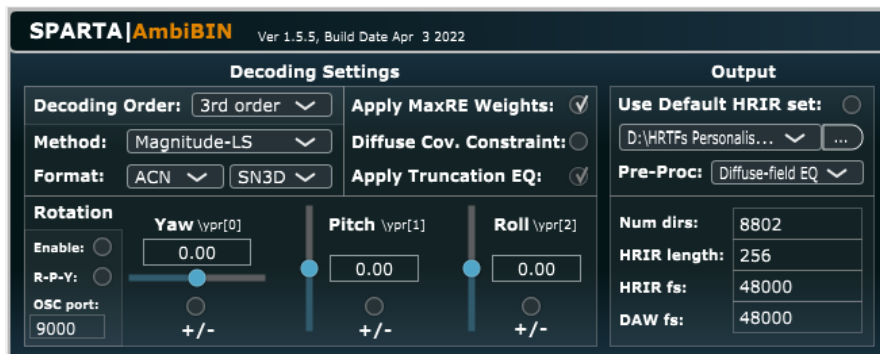
Figure 5.9: SPARTA Ambisonics Decoder converting 3rd order to 2 channel binaural audio, using the SADIE KU100, HRIR SOFA files.
