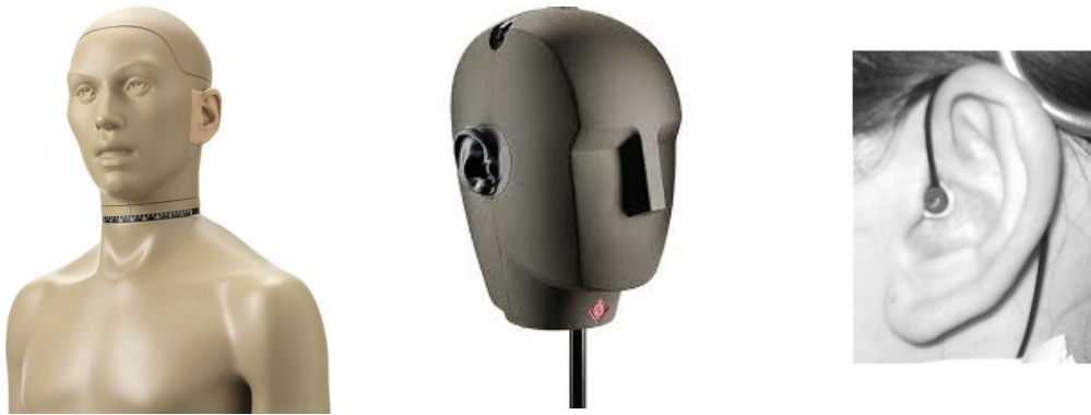
Figure 3.5: Binaural Microphones. Left: KEMAR dummy head[150]; Centre: Neumann KU 100 dummy head [151]; Right: Human Ear with locked-ear-canal measurement with miniature microphone [144].
