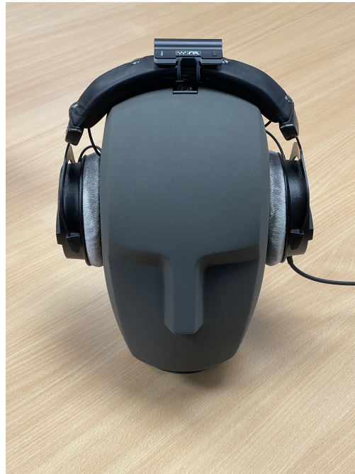
Figure 5.5: Head tracking device placed on the top-centre of the headphone band.
