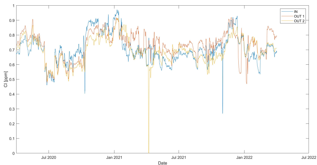
Figure 5.21: Continuous chlorine raw data from inlet and outlet monitoring at Ste 10.
