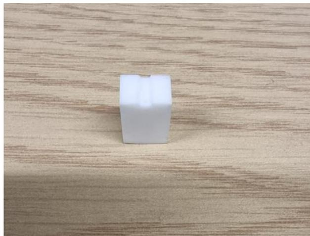
Figure 3.10: Photograph of the Rectangular DRA with a groove.
