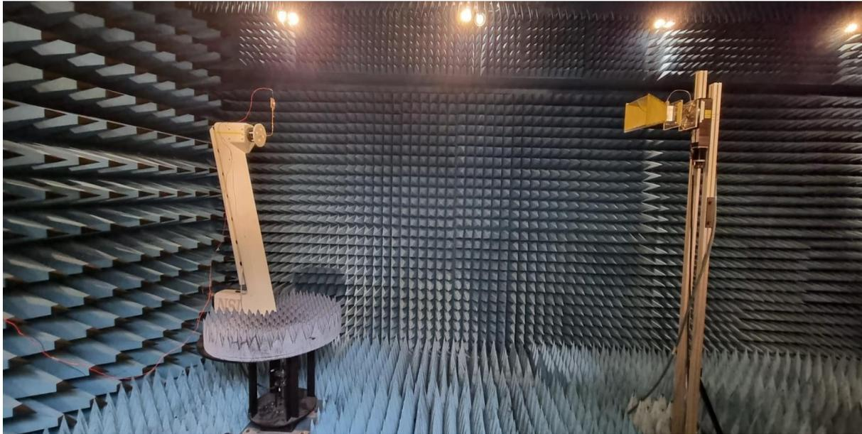
Figure 3.11: Rectangular DRA inside the anechoic chamber.
