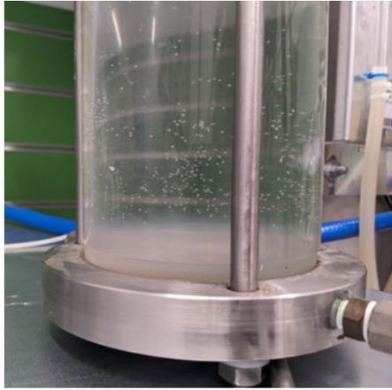
(a) Fine particles first observed at the inlet to the constant head tank (time: 48m)
