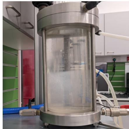
(d) The erosion front continued to move up the tank with the clear water below (time: 3 h 35 m)
