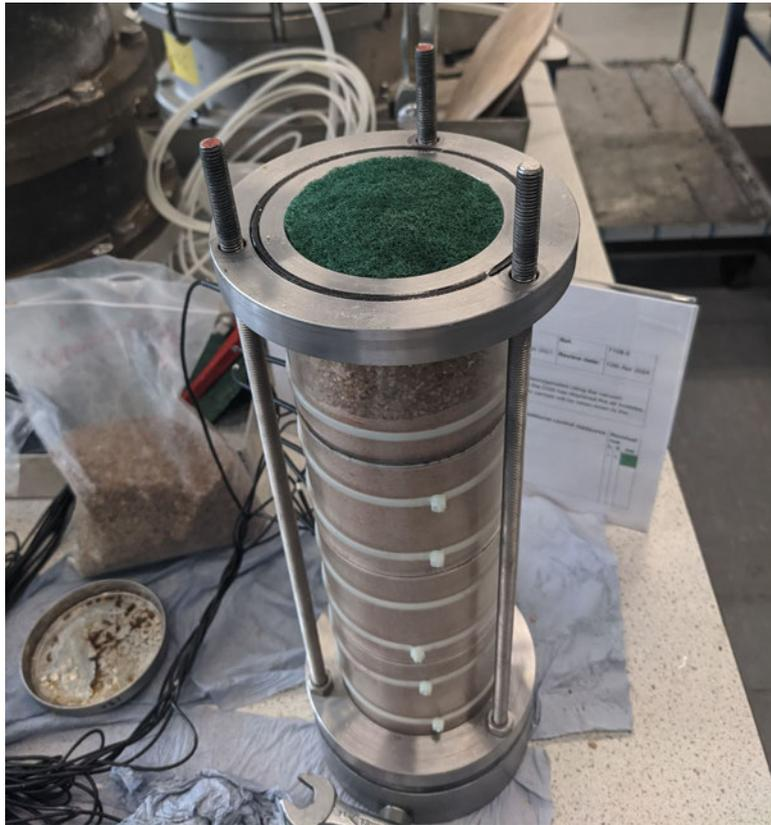
Figure 3.15: Sample is overlain with a coarse free-draining sand and a layer of permeable mesh
