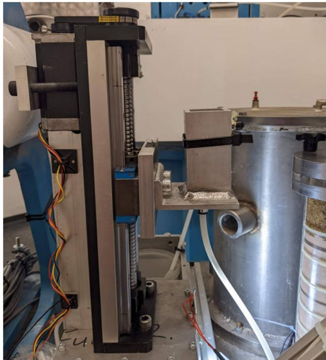
Figure 3.8: Linear actuator with stepper motor to lower the outlet CHT whilst the centrifuge is in flight
