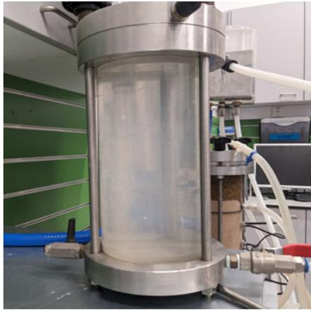
(a) Effluent water very cloudy (time: 16h 56m)
