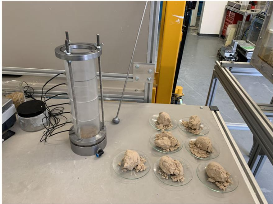
Figure 3.14: Pre-portioned layers of silt-sand soil mix are moist-tamped to their desired height in the cell
