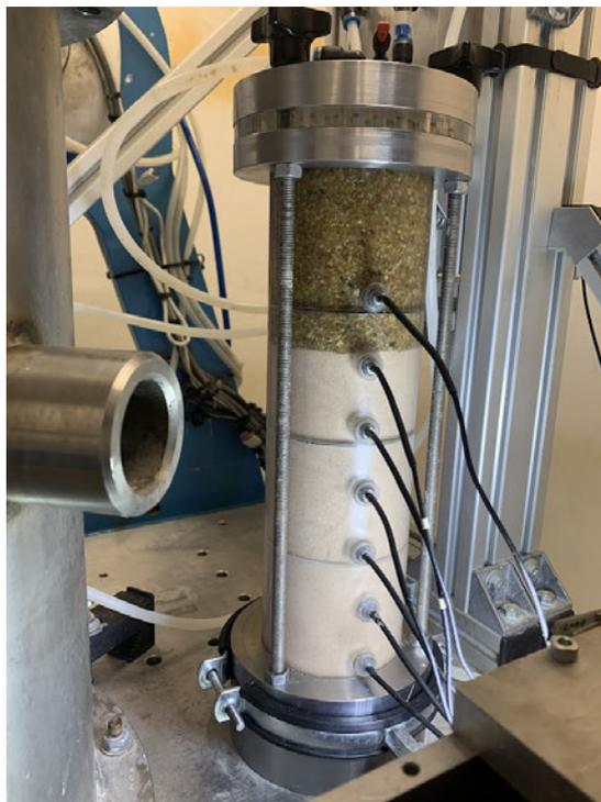
Figure 6.5: For *T20L5*, the top layer of the permeameter contained coarse sand, the specimen layers are numbered 1-5.
