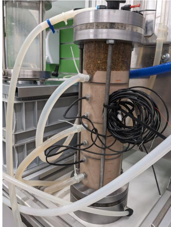
Figure 3.17: Permeameter cell measurement points modified for 1-g constant head test
