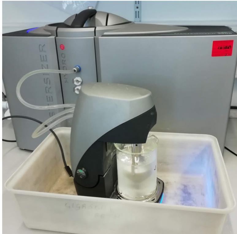
Figure 3.4: Mastersizer 3000 used to ascertain the silt particle size distribution
