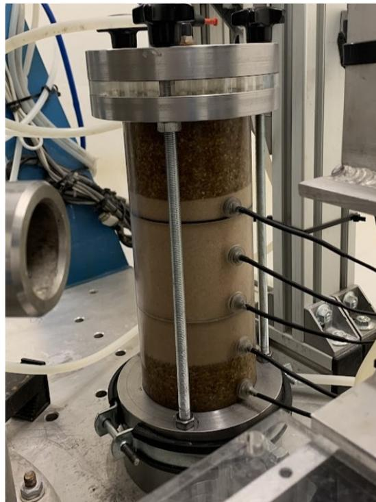
Figure 5.10: *T40S2.5* used only three of the permeameter segments to allow testing of a shorter seepage path
