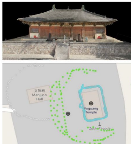
Figure 6 Top: 3D model of the Great Eastern Hall. Bottom: Camera location map of the drone and the handheld camera around the Great Eastern Hall.
