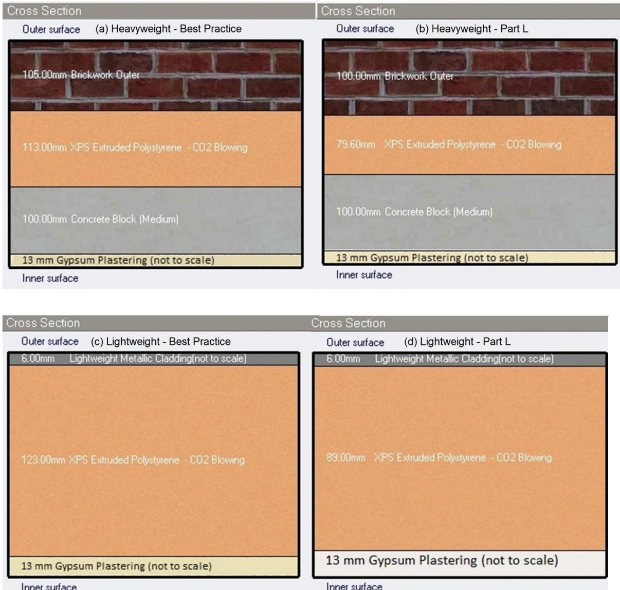
Figure A5 – External Wall construction and materials for (a) Heavyweight – Best Practice, (b) Heavyweight – Part L, (c) Lightweight – Best Practice and (d) Lightweight - Part L Building models. The layer thicknesses are not to scale.
