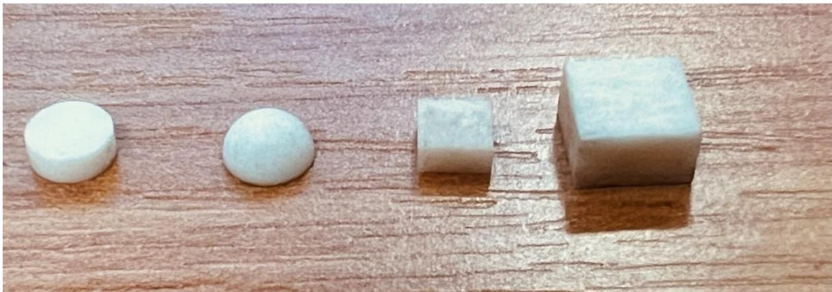
Figure 1-1 Various geometries of DR antennas.
