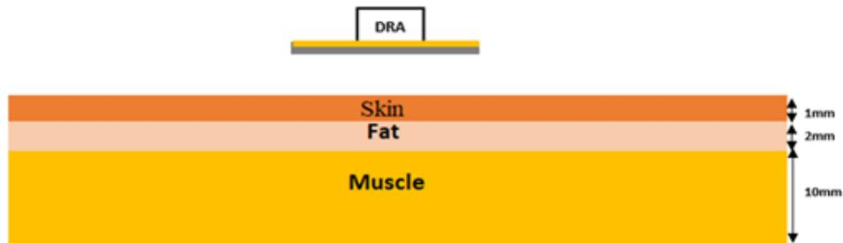
Figure 3-6. A single DRA element above the body phantom.
