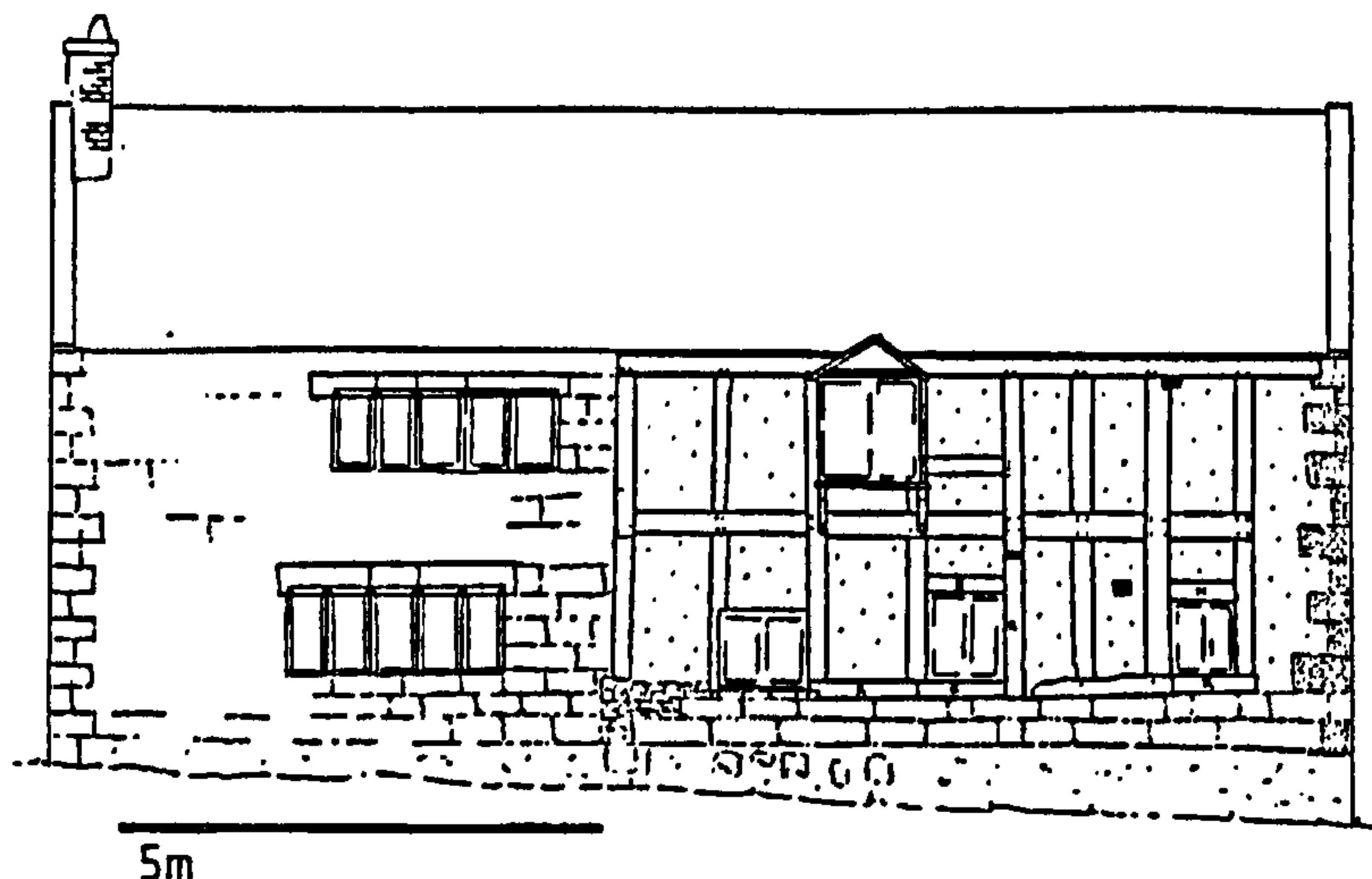
Fig. 32 Sutton House: added kitchen, 16 th century parlour wing with 19 th century gable
