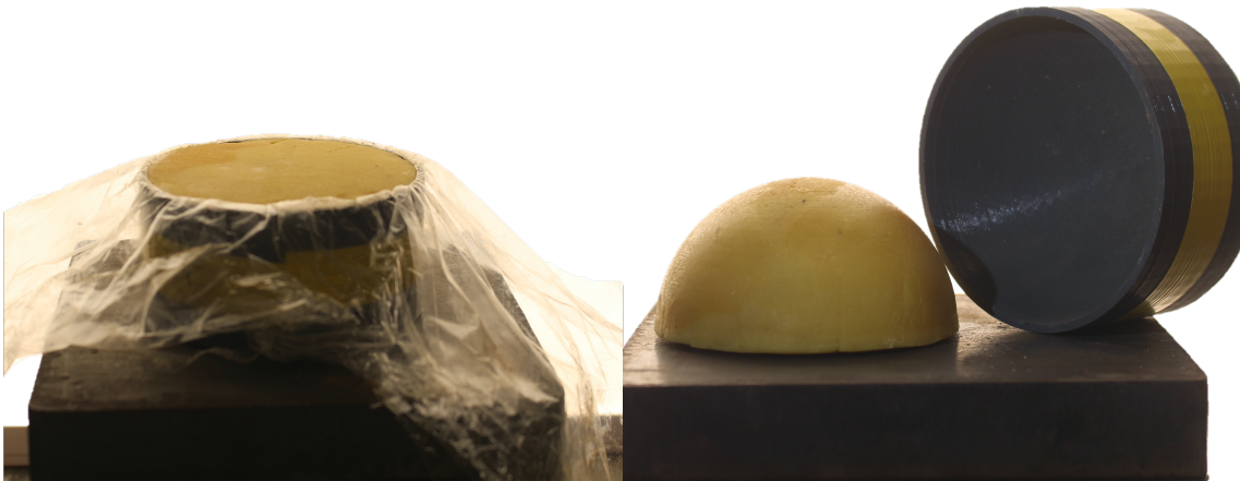
Figure 3.2: Photographs of the moulding stages of a 250g PE10 hemispherical charge in which the 3D printed mould is used to provide consistency in charge shape and density, which can be seen when removed from the casing.
