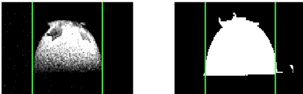
Figure 5.22: Ultra high speed video footage of a bottom detonated 250g hemispherical trial displaying the comparison between charge diameter at the time of detonation and at the point in which the detonation wave reached the charge's extents and products began to expand; this is denoted by the charge size extending passed the green lines spaced 80pixels apart in both plots.
