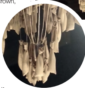
FIGURE 7: Hanging chain model of La Sagrada Família, Barcelona
