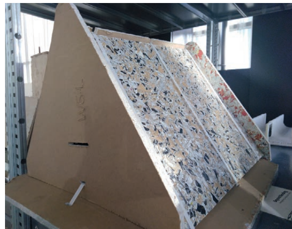
↑ FIGURE 12: Blocks made of recycled beverage carton boards, used for BRG pavilion at Ideas City Festival 2015 in New York
