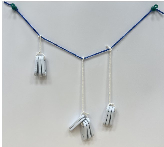
Figure 4.1: A funicular polygon generated by hanging loads on a cable or thread (in blue), the weight of which is negligible.
