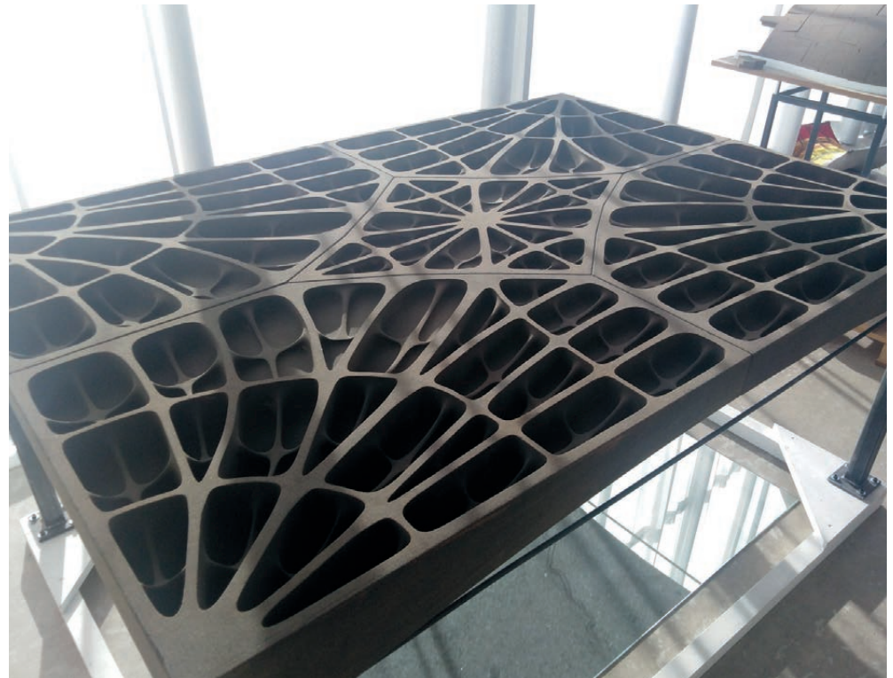
↑ FIGURE 14: 3D printed slab system developed by BRG
