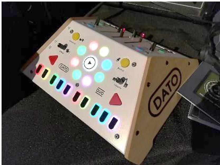
Figure 7.5. The Dato Duo synthesizer and sequencer has a two-sided design to encourage collaborative sound design and sequencing.
