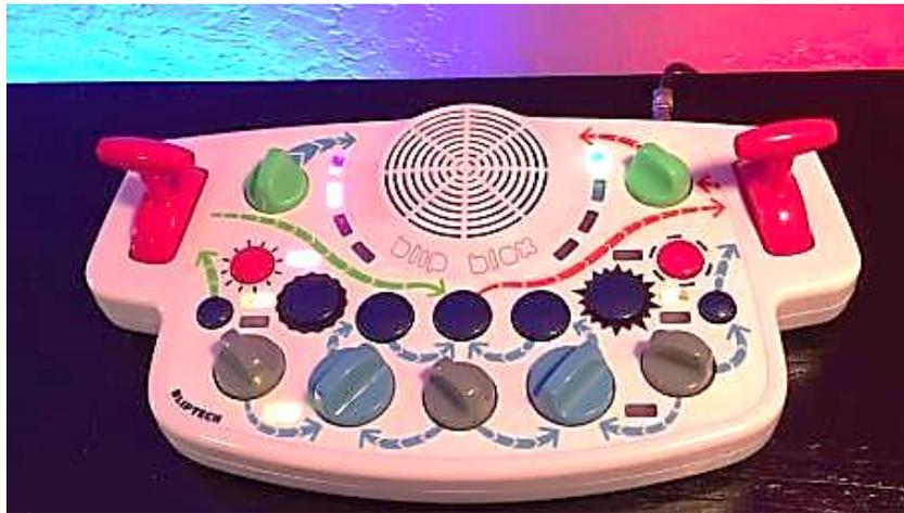
Figure 7.4. The Blipblox synthesizer has a T-bar lever on either side of its interface.
