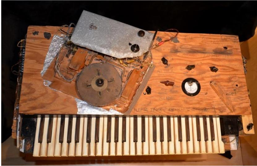
Figure 2.2. The Electronic Sackbut prototype from above.
