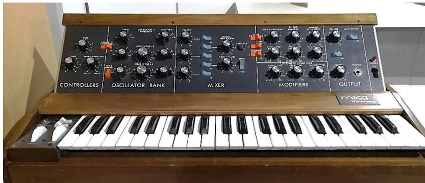
Figure 5.5. A Minimoog analogue synthesizer displayed in the MoMM, Carlsbad. This instrument utilises subtractive synthesis for generating and shaping sound.
