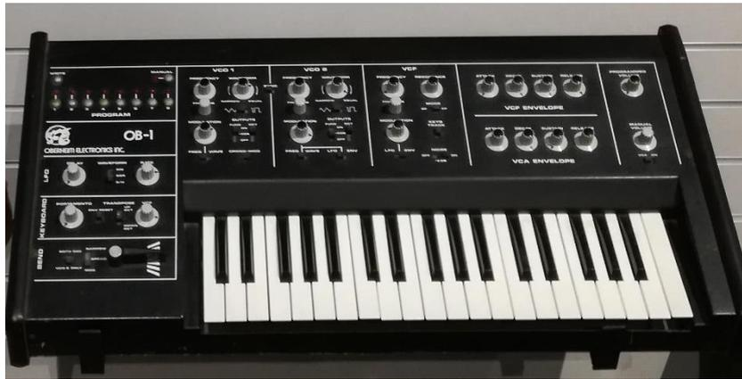
Figure 5.6. An Oberheim OB-1 displayed in the MoMM. Two waveforms are provided for each of its two oscillators, as symbolised by triangular and square shapes.
