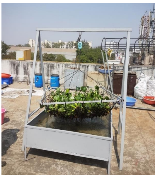
Plate 3.2-3: Weighing water hyacinth mat in large tank with net and pulley system (February 2020).
