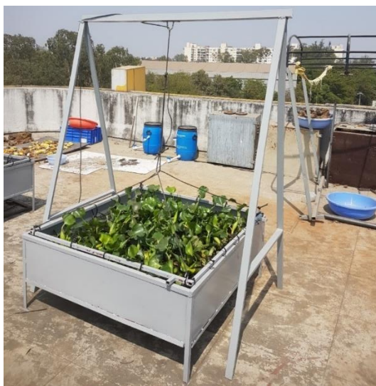
Plate 3.2-2: Large tank with net and pulley system (February 2020).
