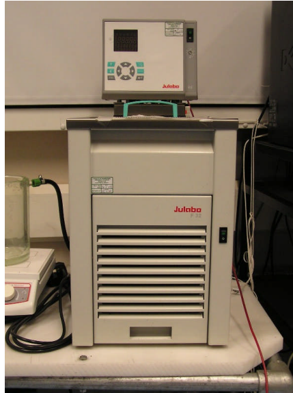
Figure 3.6: Julabo refrigerated and heating circulator (F32-HE)
