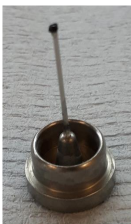
Figure 4-2 Photographic image of biochar sample SCG350 mounted to a pin and magnetic contact for tomographic image acquisition
